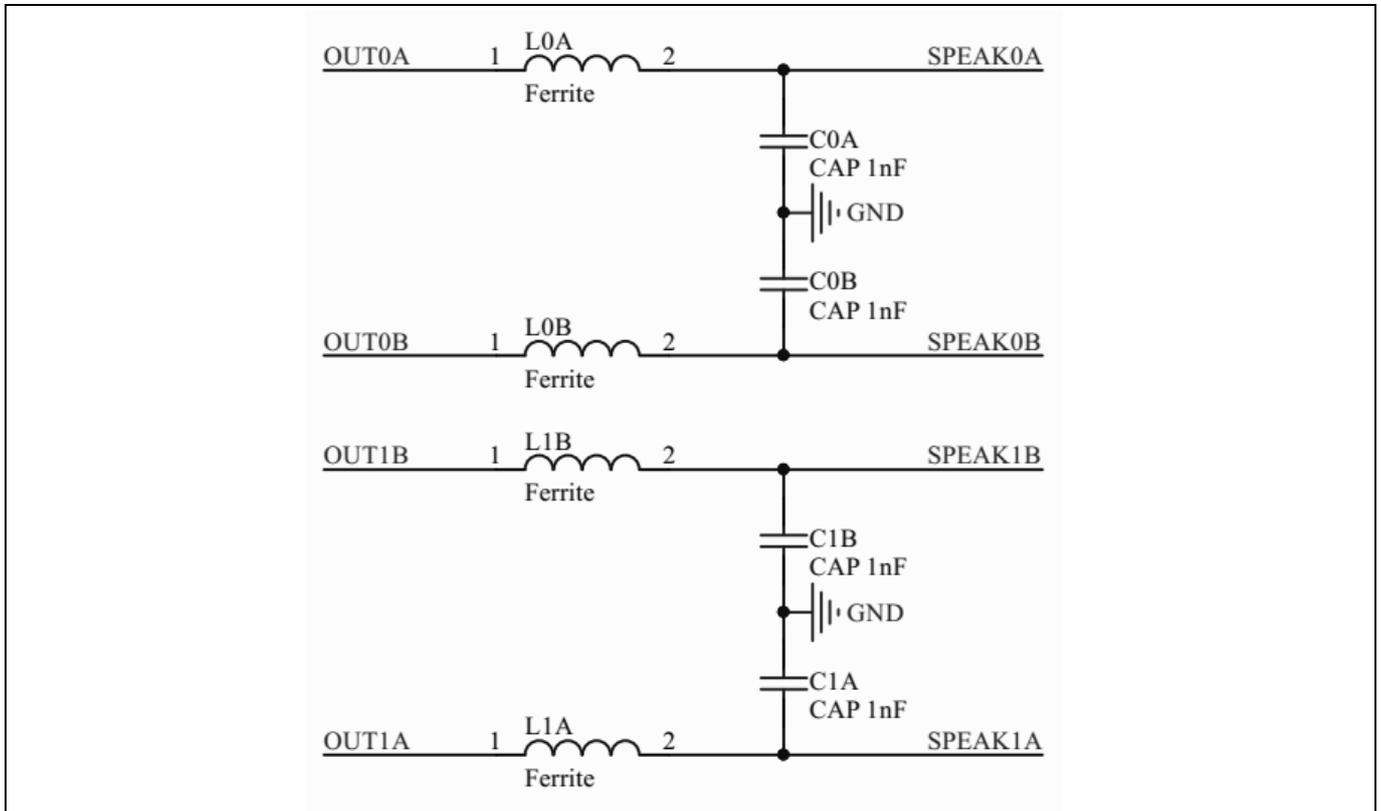
**Figure 2** Typical ferrite filter for 2xBTL output for MA120xx(P) amplifiers
