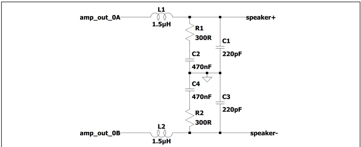
**Figure 5** LC output filter configuration 2 with damping filter for 1x BTL output
