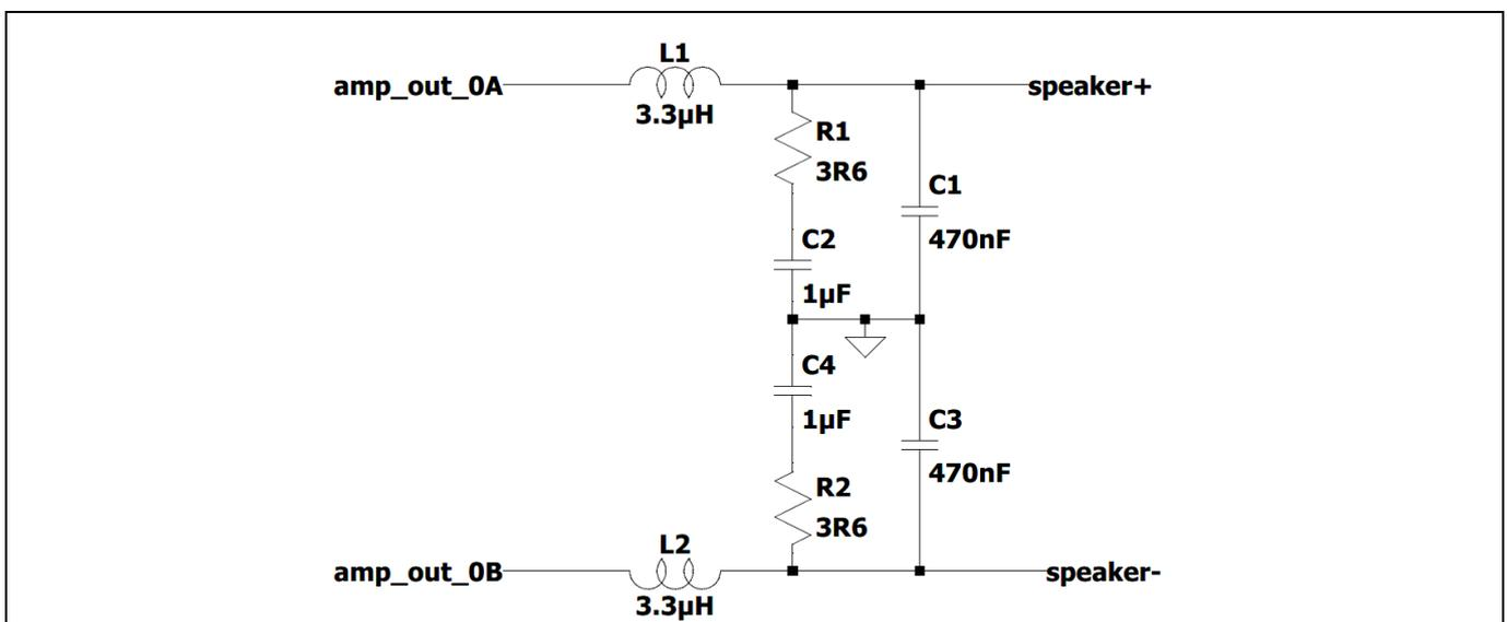
**Figure 4** LC output filter configuration 1 with damping filter for 1x BTL output
