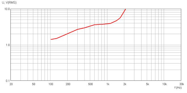
The curve maximum RMS voltage at low frequencies.
