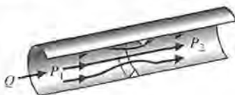
FIGURE P2.5 Flow through an orifice.
