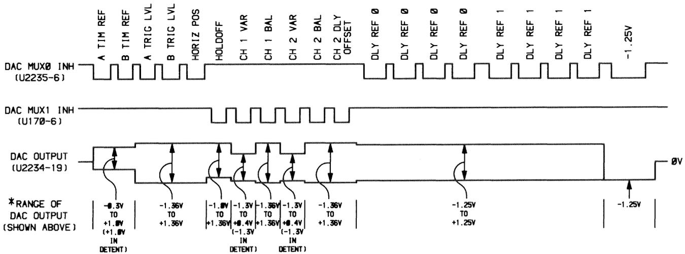
\*NOTE: AS ANY GIVEN CONTROL IS EXERCISED, THE CORRESPONDING PORTION OF THE DAC OUTPUT WAVEFORM SHOULD VARY WITHIN THE LIMITS INDICATED.
