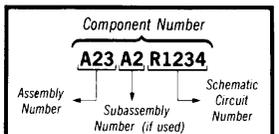
Chassis-mounted components have no Assembly Number prefix—see end of Replaceable Electrical Parts List.
