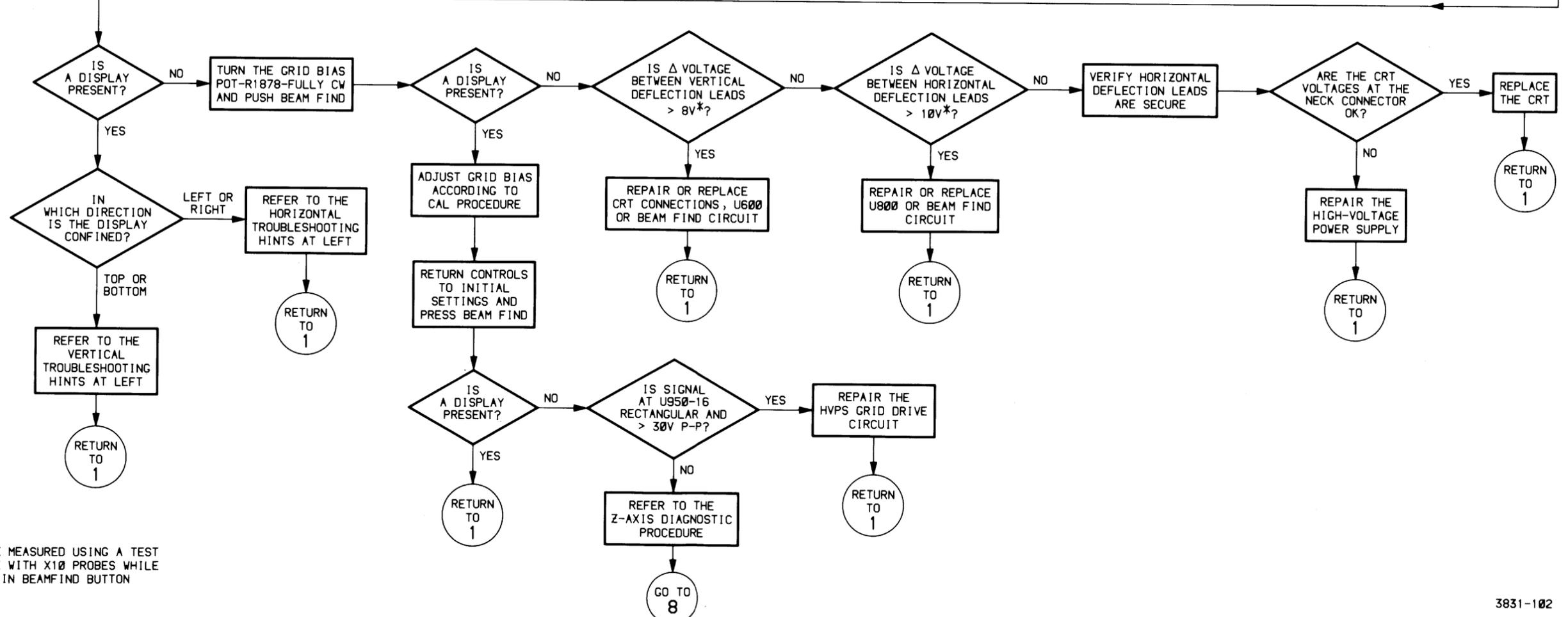
\* VOLTAGES ARE MEASURED USING A TEST OSCILLOSCOPE WITH X10 PROBES WHILE HOLDING IN BEAMFIND BUTTON
