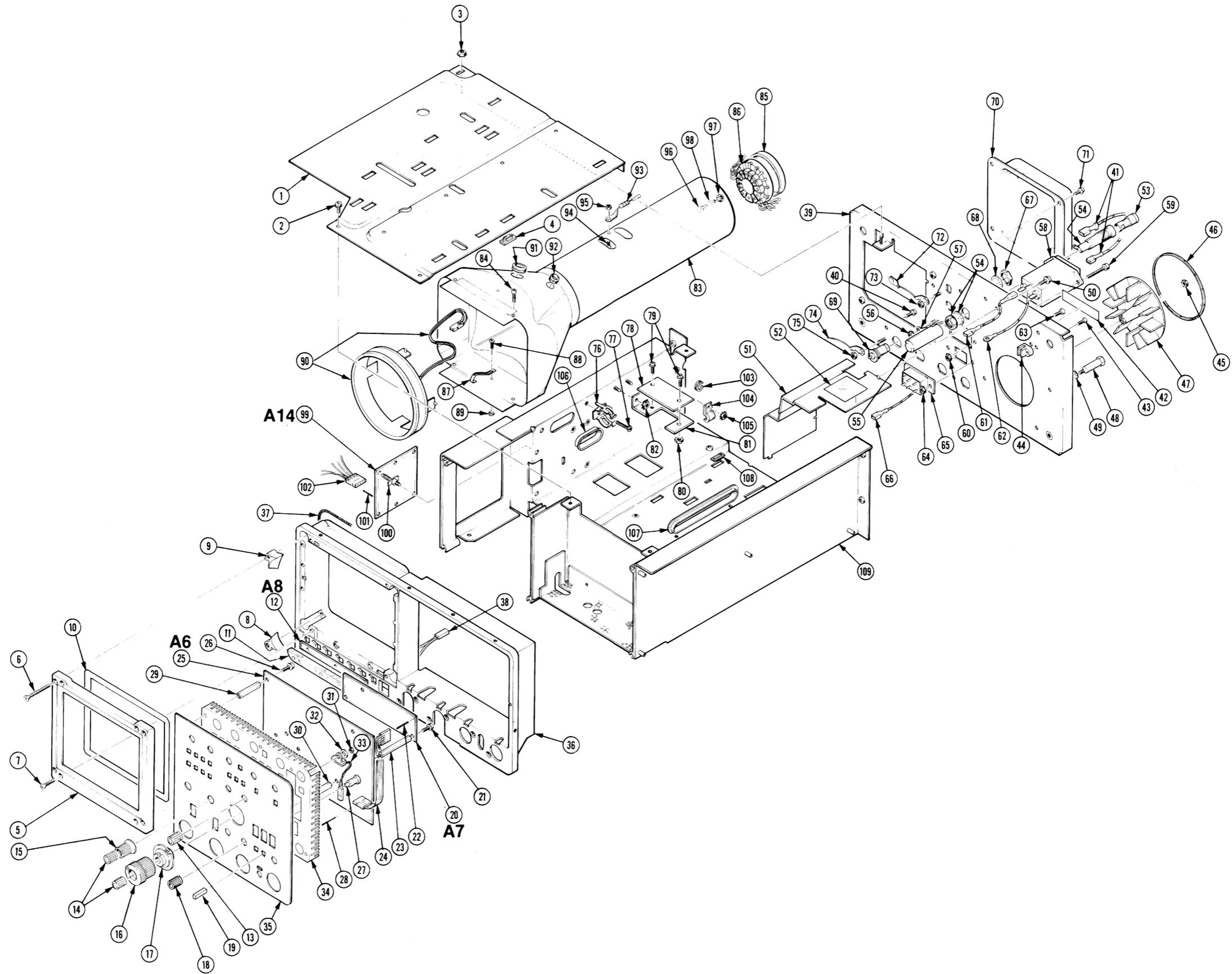
Replaceable Mechanical Parts—2465 Service
