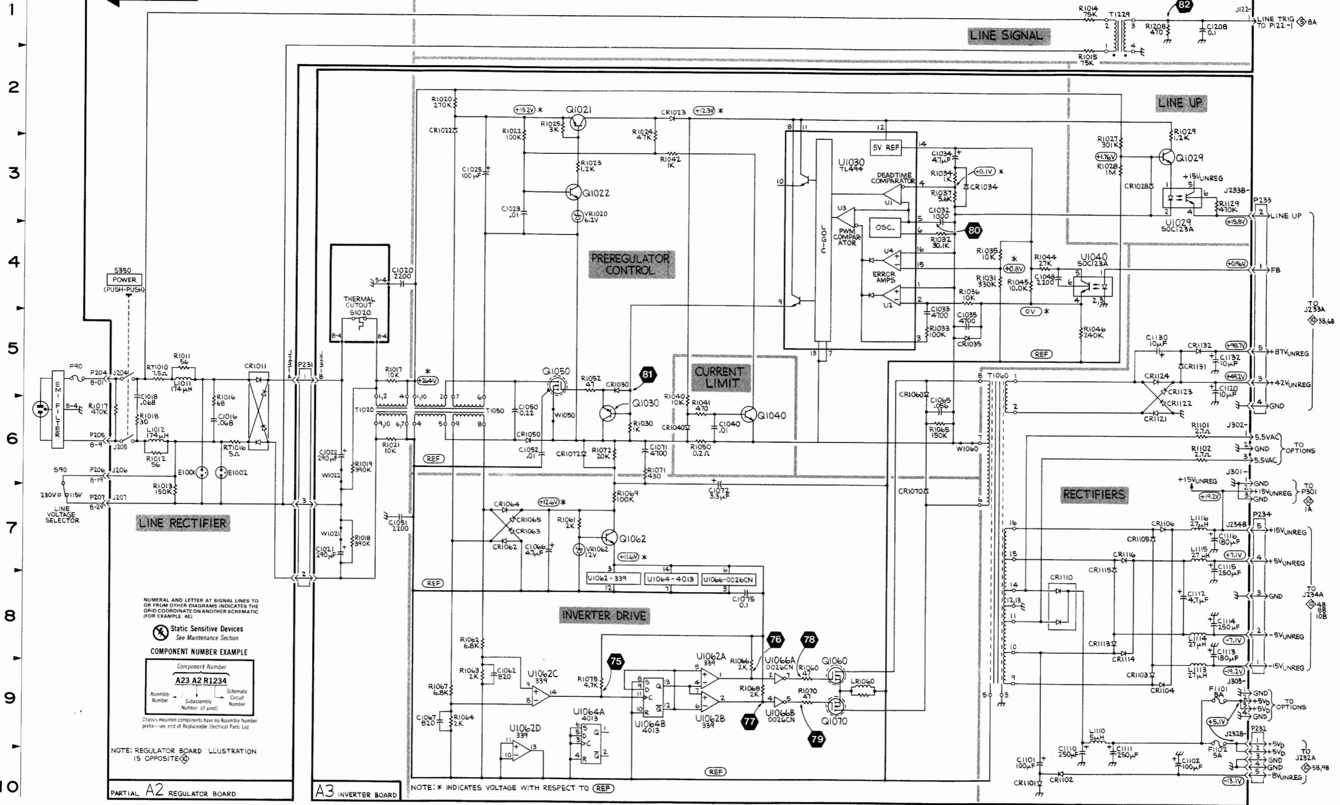
NUMERAL AND LETTER AT SIGNAL LINES TO OR FROM OTHER DIAGRAMS INDICATES THE GRID COORDINATE ON ANOTHER SCHEMATIC (FOR EXAMPLE: 4E)
