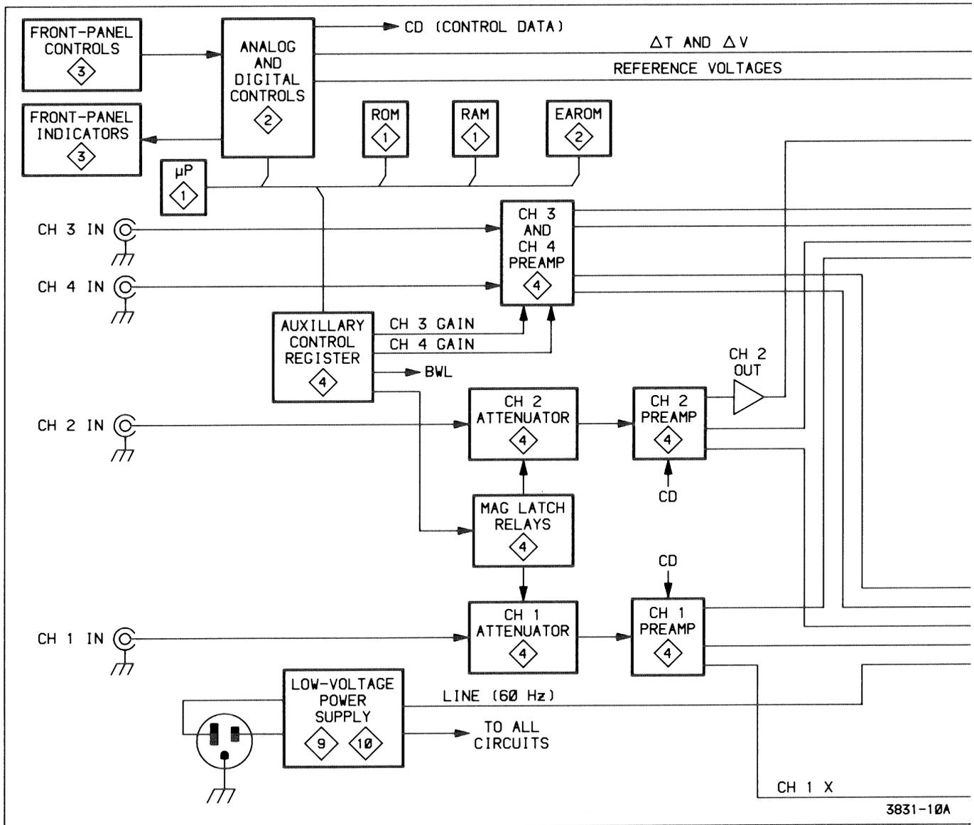
Figure 3-1. Block diagram.
