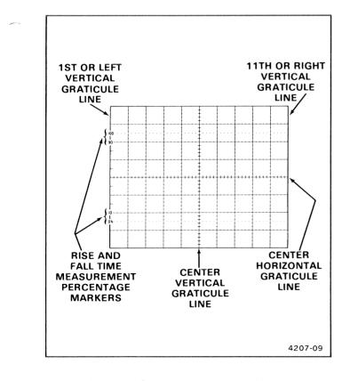
Figure 2-9. Graticule measurement markings.
