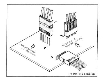
Figure 6-1. Multipin connector orientation.
