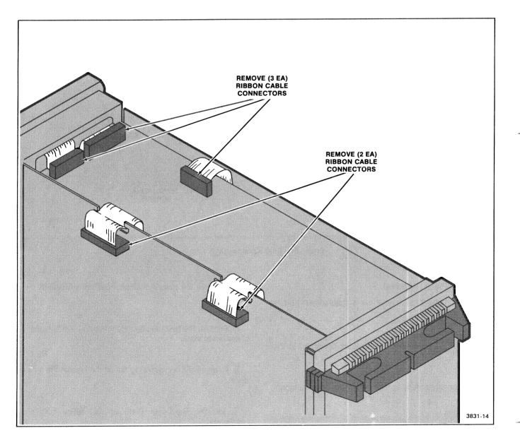
Figure 6-3. Ribbon cable removal.
