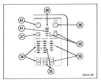
Figure 2-6. Trigger controls and indicators.
