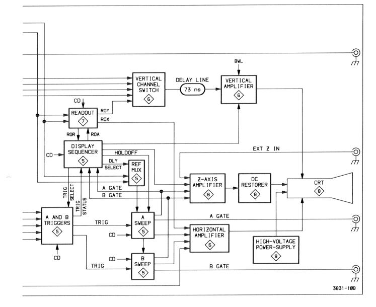
Figure 3-1. Block diagram (cont).
