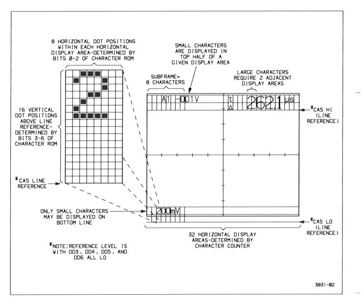
Figure 3-7. Developing the readout display.
