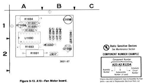
Figure 9-13. A10—Fan Motor board.
