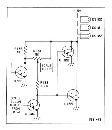
Figure 3-5. Scale Illumination circuit.
