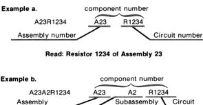
Read: Resistor 1234 of Subassembly 2 of Assembly 23
