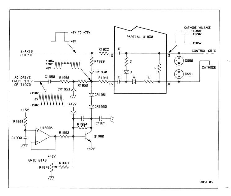
Figure 3-10. Dc Restorer circuit.
