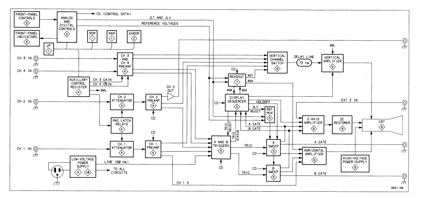
Figure 9-4. 2465 block diagram.
