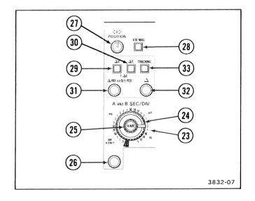
Figure 2-5. Horizontal and delta measurement controls.
