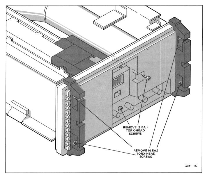
Figure 6-2. Rear panel removal.
