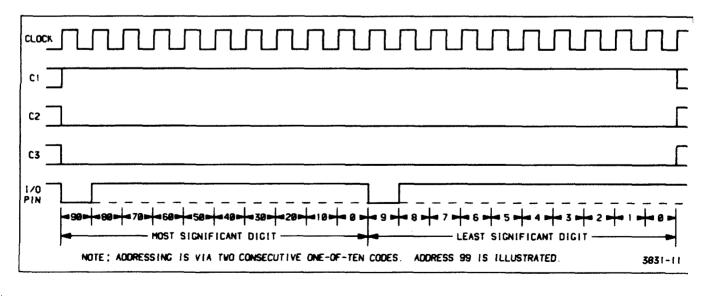
Figure 3-3. Accept address timing.
