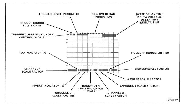
Figure 2-8. Readout display locations.
