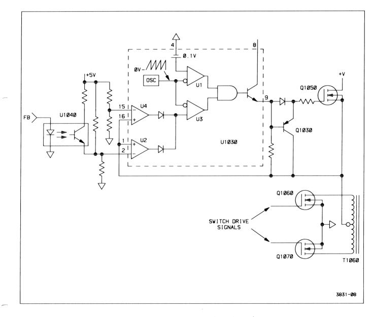
Figure 3-12. Simplified schematic of control network.
