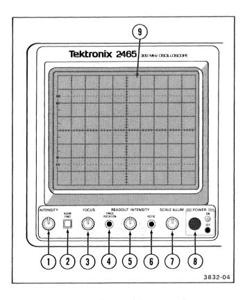
Figure 2-2. Power and display controls.
