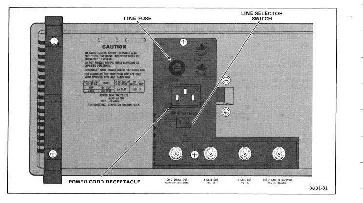
Figure 2-1. Line selector switch, line fuse, and detachable power cord.
