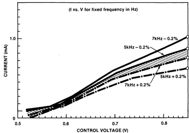
Figure 4. I (V) Converter Curve Variations Causing ± 2% Dolby Transfer Curve Error
