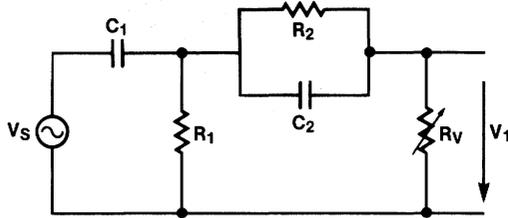
**Figure 15. Side Chain Filter**
