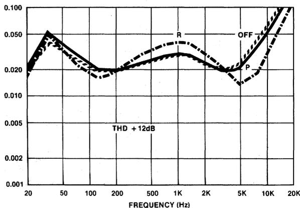
Figure 13. Distortion Plus Noise at +12dB Input
