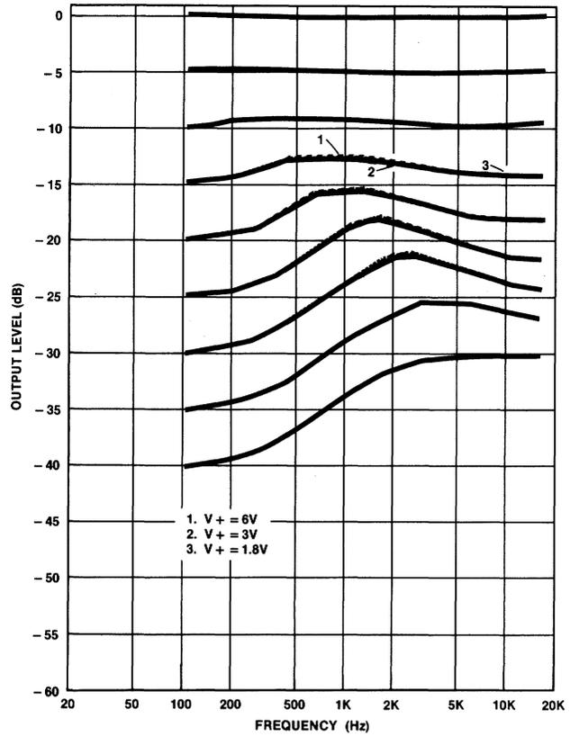
Figure 14. Amplitude Response Variations with Power Supply Voltage
