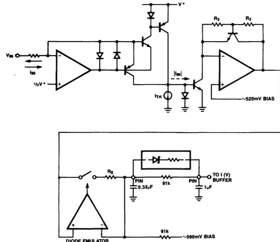
**Figure 8. Full Wave Rectifier and Attack/Decay Circuit Concept**
