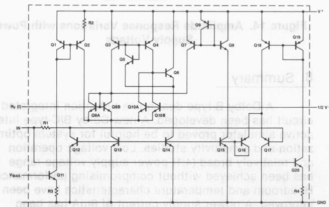
Figure 10. Voltage-to-Current-to-Resistance Converter
