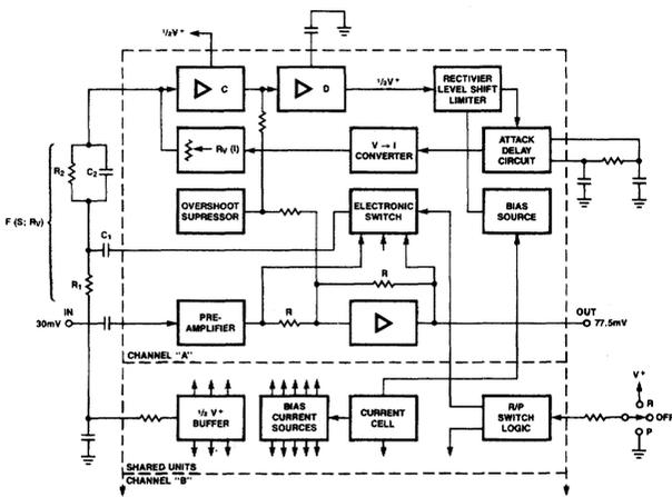
Figure 2. Block Diagram of the Dual Record/Play IC
