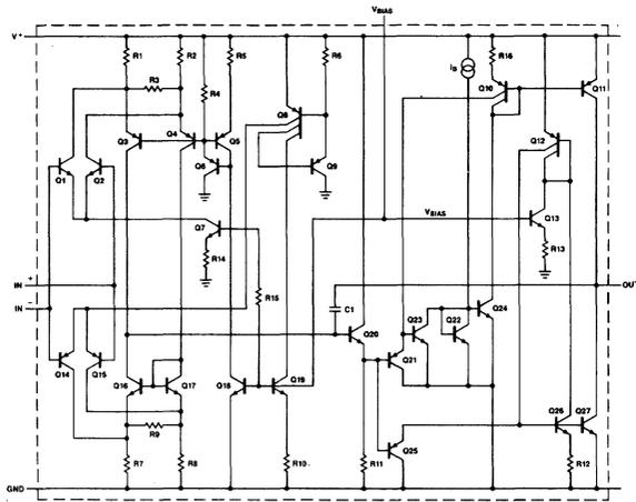
**Figure 6. Operational Amplifier with Rail to Ground Input/Output Swing**
