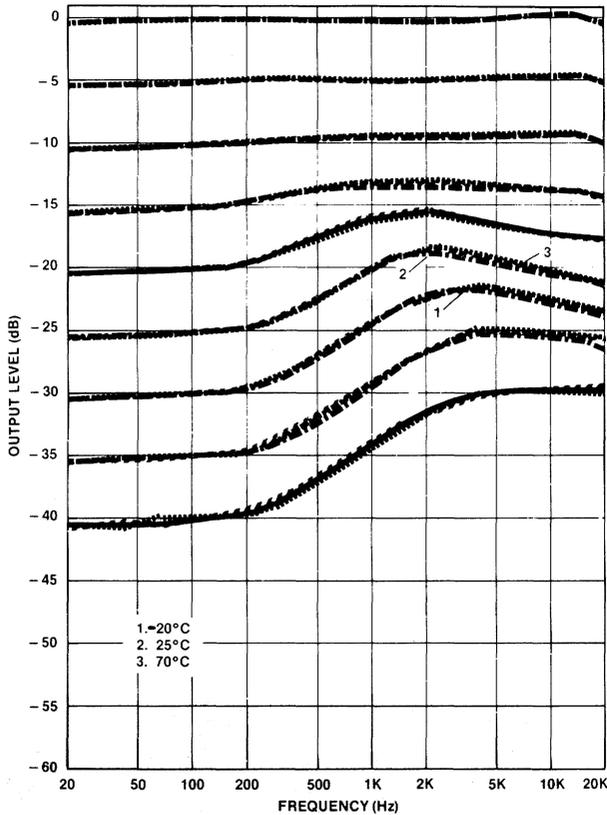
Figure 12. Amplitude Response Variations with Temperature
