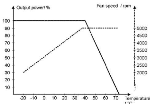
Output power and fan speed / ambient temperature
