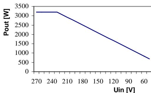
Output power / input voltage de rating curve
