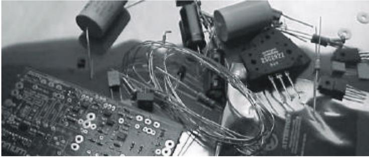
Start by mounting the lowprofile components, like resistors and trimmers. Follow the printed values on the PCB itself, and compare with the color codes printed on the previous page. If You are sure everything is mounted correctly, solder it down. After this fit the capacitors, first the smaller ones and then the larger ones. Solder.
