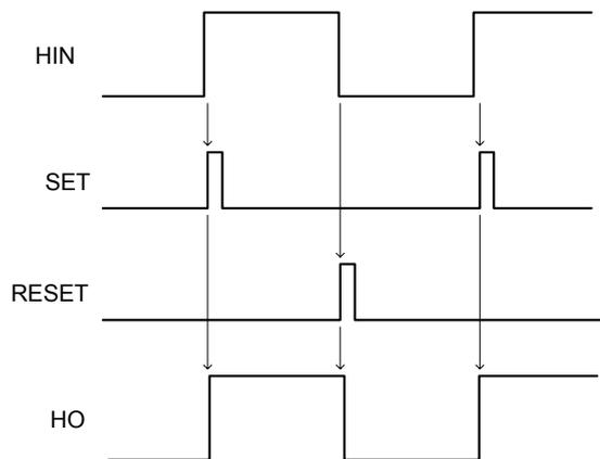
The high-side circuitry reconstructs PWM from SET and RESET pulses.
