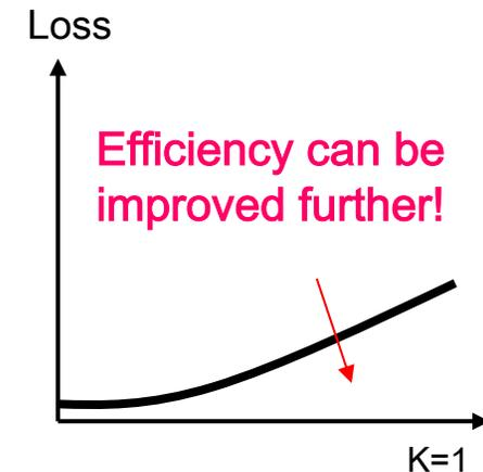
K is a ratio of Vbus and output voltage.
