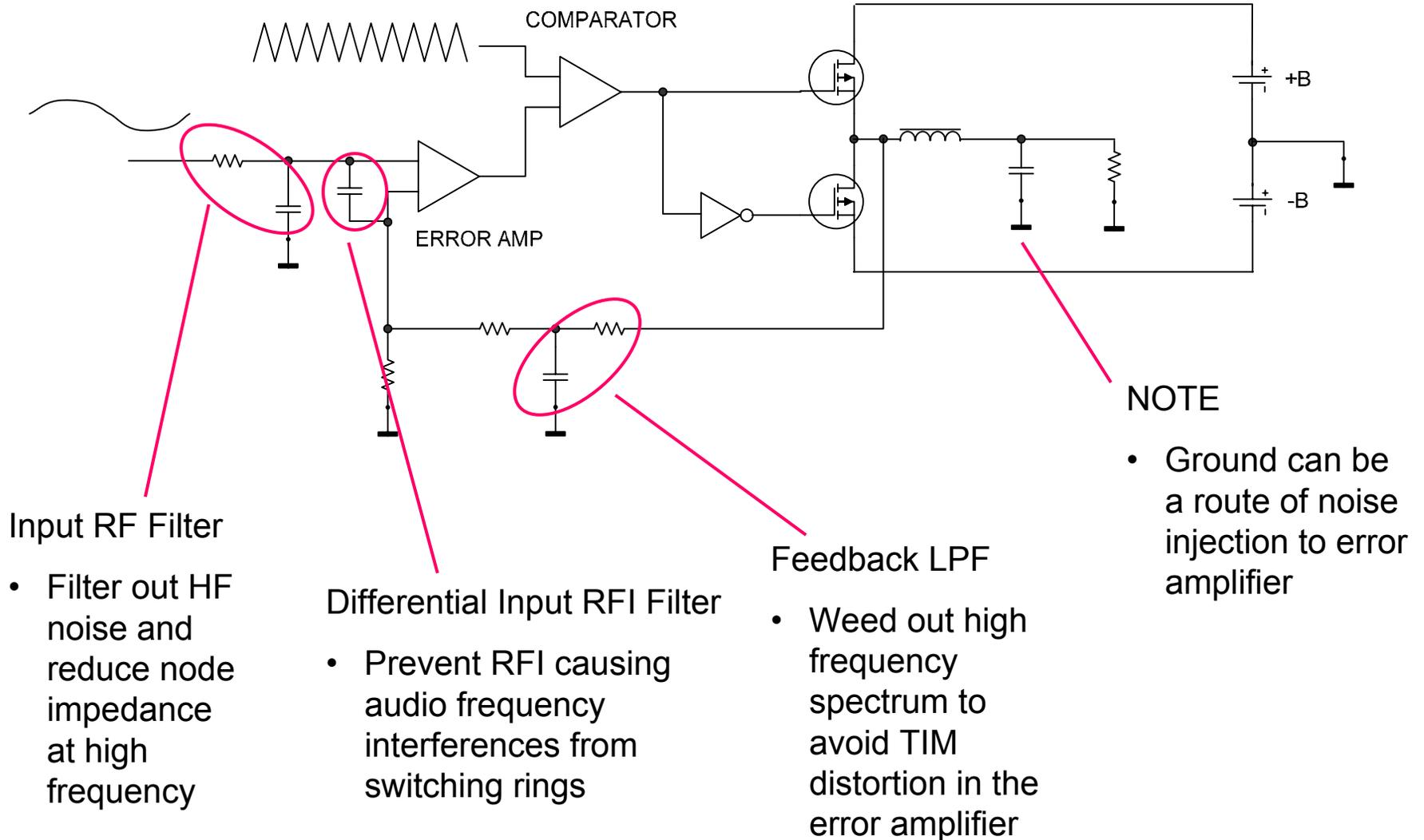
Analog stage uses non-linear components such as diode, BJT and FET.
