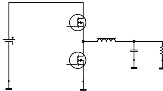
$$V_{IN} \times I_{IN} = V_{OUT} \times I_{OUT}$$
