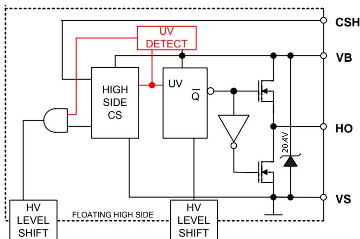
**UVLO of VBS shuts down HO and disable high-side current sensing**
