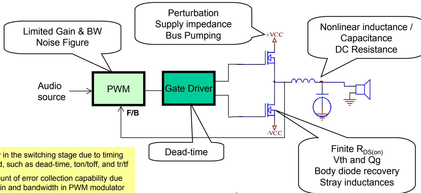
1. Non-linearity in the switching stage due to timing errors added, such as dead-time, ton/toff, and tr/tf
