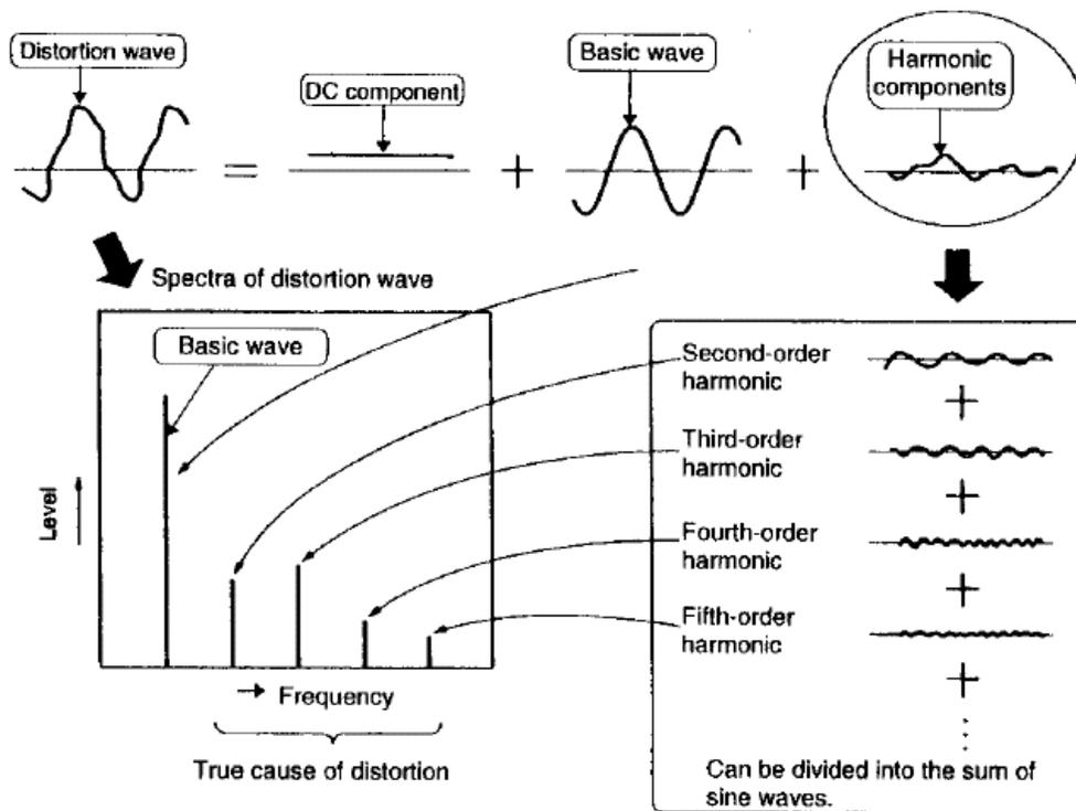
Any repetitive waveforms can be expressed as a sum of sinusoidal signal as
