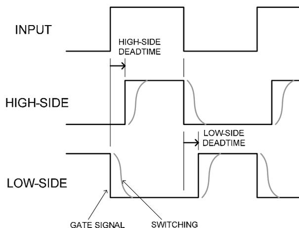
Dead-time (or blanking time) is a period of time intentionally inserted in between the ON states of high- and low-side MOSFETs.
