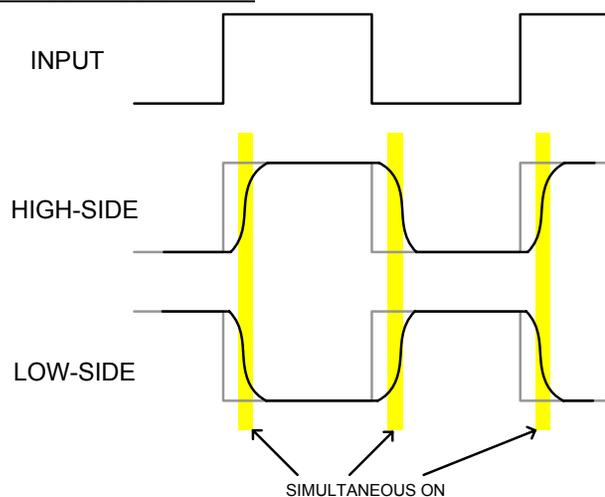
Lack of dead-time results in lower efficiency, excessive heat and potential thermal failure.
