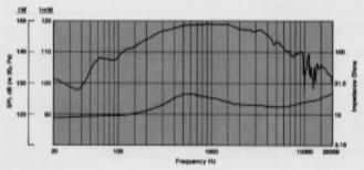
Frequency response and impedance modulus of Model 2445J coupled to a 49 mm (2 in) diameter terminated plane-wave tube, with sensitivity referenced to a 25 mm (1 in) tube. This is the power response of the transducer, and is the frequency response that will be obtained on a true full-range constant directivity horn design, such as JBL's 2360 series of Constant Coverage Bi-Radial Horns.
