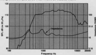
Frequency response of the 2445J coupled to a JBL 2380 Flat-Front Bi-Radial horn, measured on-axis at a distance of 1 meter with a 1-watt (4.0 V RMS) input in a reflection-free environment, with impedance vs. frequency curve. A horn with a pure exponential flare, such as typical radial horn designs, will exhibit greater high frequency output on-axis at the expense of lost annular coverage.
