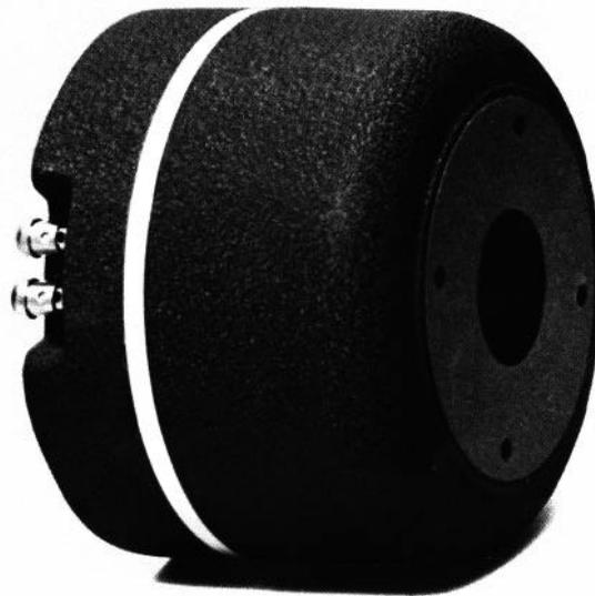
Model 2441 is a powerful, professional-quality compression driver built to typical JBL standards of precision. Featuring a 100 mm (4 in) voice coil and an Alnico V magnetic structure weighing more than 10 kg (23 lb), it can take the most explosive transients in stride and reproduce them at thunderous levels with flawless accuracy.
