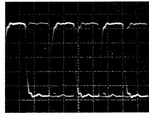
39 IC362 4pin (LRCK) 5.6Vp-p, 0.52μs
