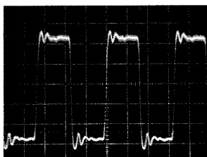
25 IC307 58pin (F128) 5.8Vp-p, 0.17μs
