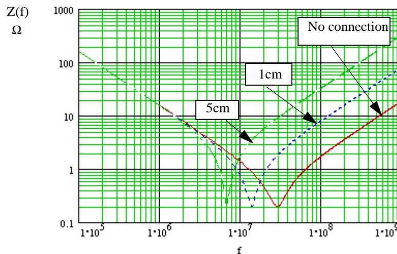
Figure 21. Connexion increase the impedance in H.F
