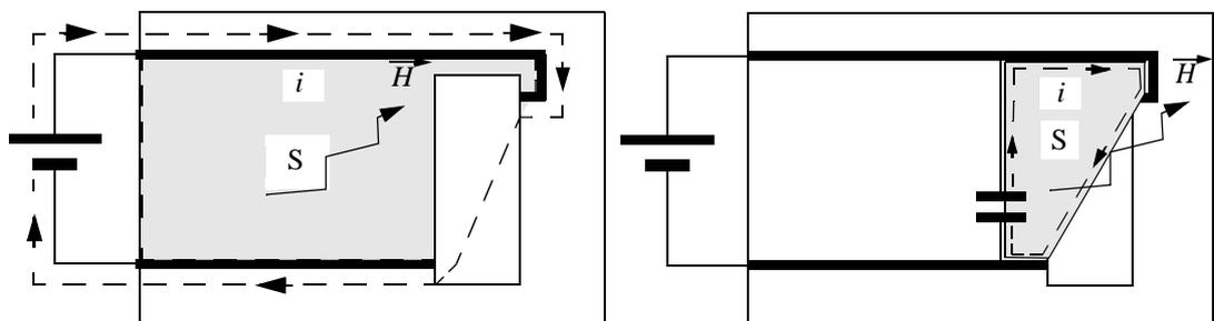
**Figure 4. Decoupling capacitor reduces the magnetic field and the loop surface.**
