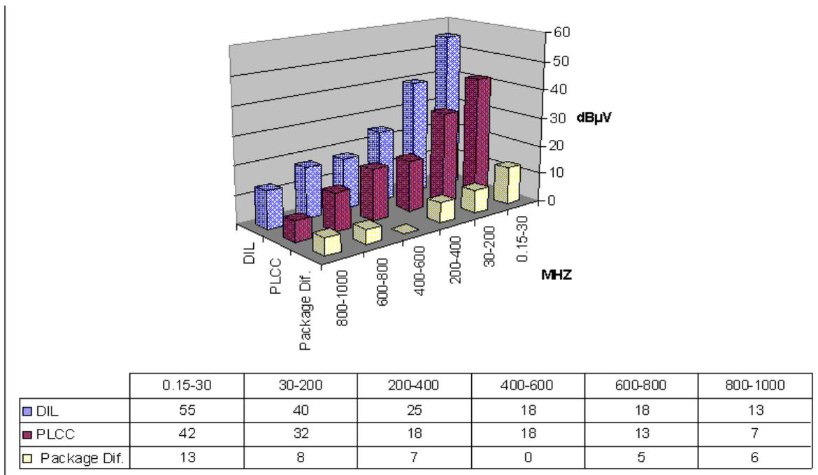
**Figure 23. Package effect on the radiated emissions**
