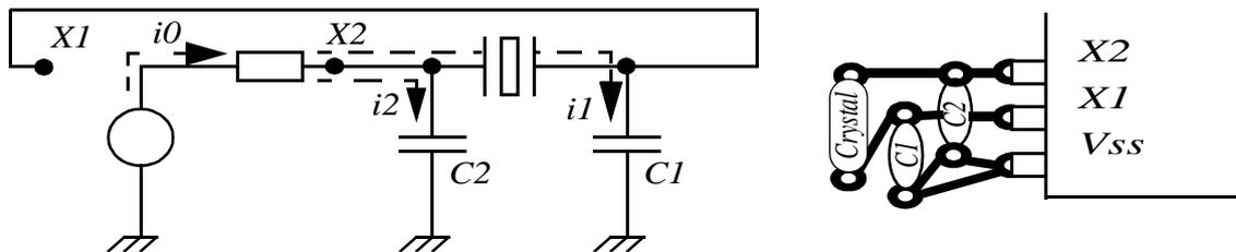
Figure 9. Oscillator lay-out
