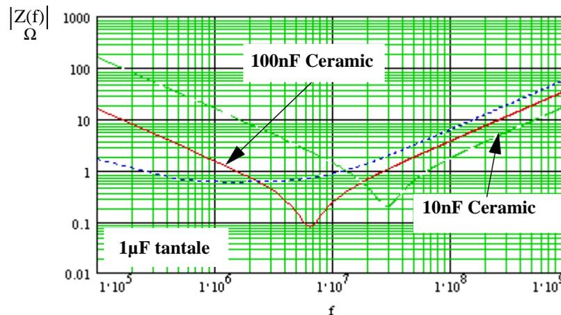
**Figure 19. Plots versus frequency of several types of capacitor**
