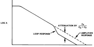
Figure 3b. Response of circuit 3a, neglecting R<sub>OUT</sub>. Pole- Zero mismatch may yield poor transient response.
