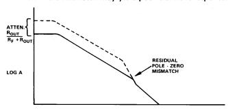
Figure 3c. Response of circuit 3a with finite ROUT.
