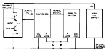
Figure 11. Improved ground current management (analog and digital common must be joined in either converter or analog system. Diodes are fault protection if this connection is broken.)
