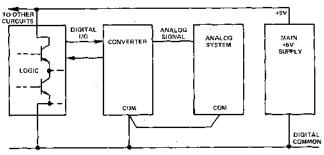
(b) This connection minimizes common impedance between analog and digital (including converter digital currents).
