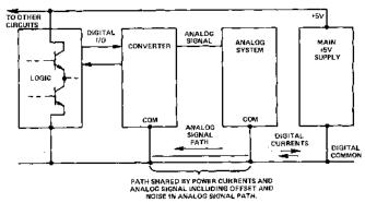
(a) Shared path produces interference and errors.
