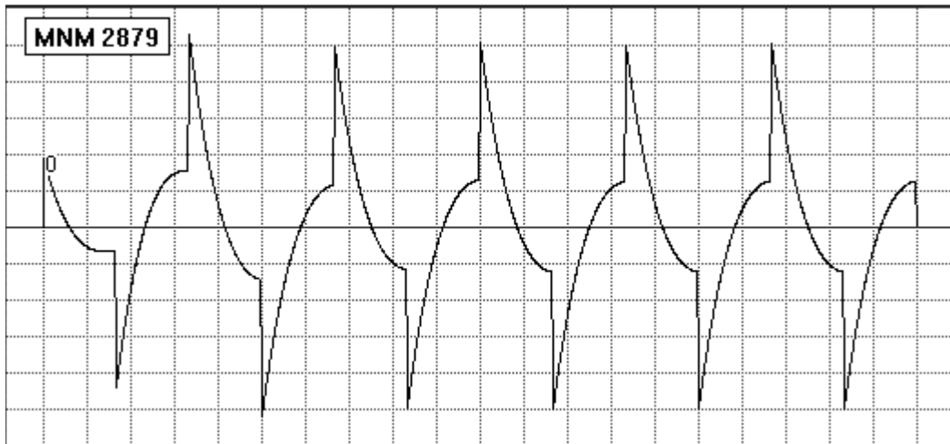
Figure 2. Resopnse of the system shown in Figure 1 to a 100 Hz square wave input.
