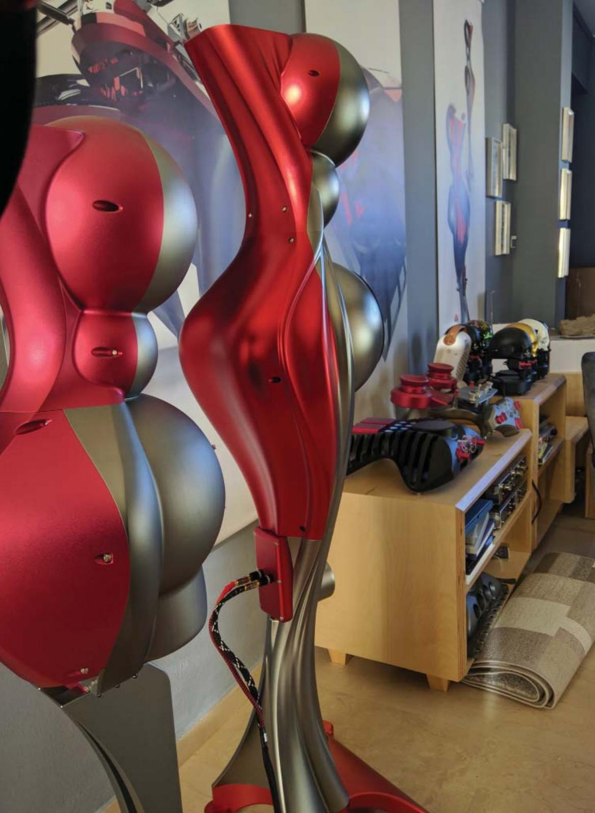
Using ideas borrowed from Neumann TLM 50 and M150 microphones, the SIREN embeds the Accuton drivers into spheres mounted onto an organic “time-aligned” sculpture. Despite the unique and unusual shape, the design is a seriously engineered, no-compromise loudspeaker with emphasis on absolute sound quality.
