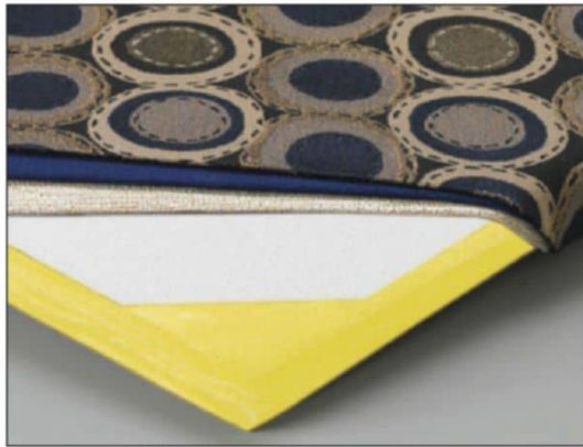
Photo 2: A thin hardened layer of fiberglass under the cloth adds impact resistance and improves low-frequency absorption.
