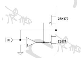
Since the opamp reduces the input impedance by some 80dB at 1kHz or below, one can now consider using other JFET pairs such as 2SK246BL/2SJ103BL with essentially the same distortion performance, but with somewhat increased noise ( $\sim 2nV/\sqrt{Hz}$  at input). These JFETs, without the
