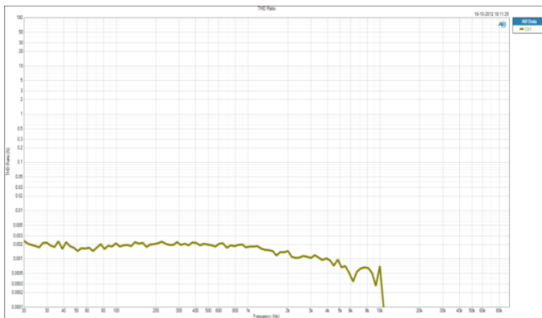
Figure 6 THD ratio vs. Frequency. Measured with 0 dBV output signal. THD ratio approximately 0.002% across audio band.
