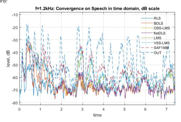
... and we start to see that long echo tail is detrimental to VSS-LMS and plain LMS: the residual error signal exceeds the OUT signal due to misbehaving echo tail (around 3 sec).
