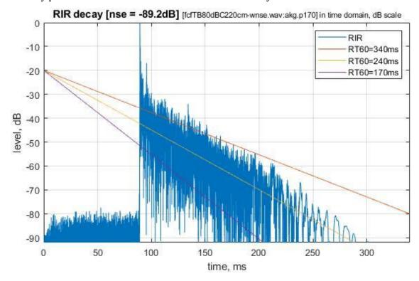
There is no white [modelling] noise at the RIR tail [as in MLS or Sine Sweep cases] obscuring the reality which is a special beauty of kernel-based System Identification approach.
