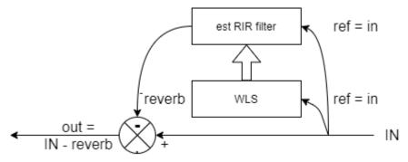
Let's investigate how it works using a simple model, without any additional complications like subband decomposition, etc.
