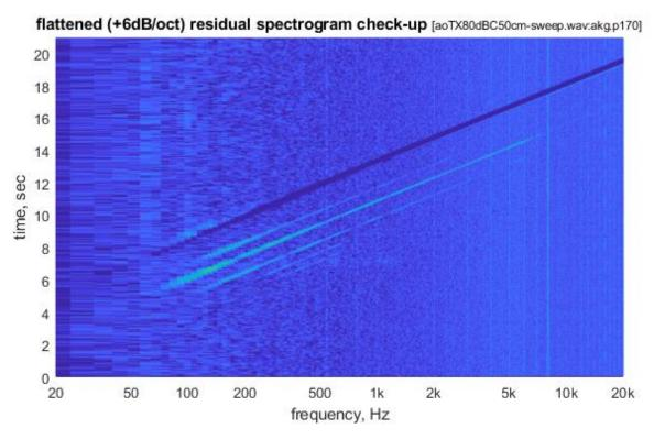
The residual spectrogram shows how strongly SineSweep RIR measurement method is sensitive to the noise: see the 0.5sec deep blue trench immediately after the chirp. This can be alleviated by making multiple passes, as for MLS – which, however, may take too much time because you cannot shorten the chirp without losing resolution.
