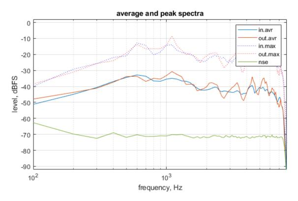
Now we can apply subband decomposition with less fear that aliased powerful low frequency noise may spill over weak high-frequency components. We use 80 bands for 16kHz sampled signals, with long (L=16) asymmetric LD (latency=5) filterbank.
