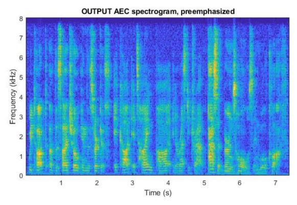
Here we see formant structure, voiced and unvoiced sounds, pauses before stop consonants (plosives), on a background of white noise, with average SNR of 30...35dB, peaking to  $\sim 60$ dB.
