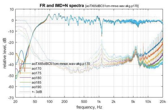
The seemingly illogical MNSE IMD+N rise above 6kHz is proper – distortions drop below the noise floor.
