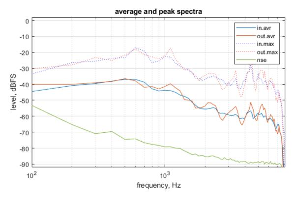
The voice is also 1/f after 500Hz, so the first signal processing operation we do is a spectral flattening with a 1st order IIR filter, the same for both IN and OUT, to be reversed by inverted IIR on RES.
