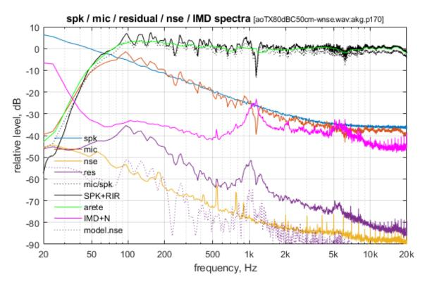
The FSAF residual's PSD is higher than for SineSweep and MLS. AWGN has higher peak to average ratio (~12dB vs 3dB). The AWGN signal in LADF-dimensional space looks like a ball of fog a full-dimensional
