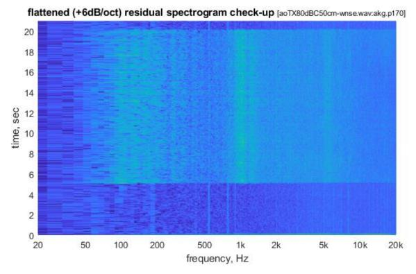
The FSAF residual' spectrogram is non-stationary at f > 10kHz, the lowest in the middle of excitation due to the ribbon tweeters' power [mis]handling. The tweeter efficiency is  $\sim$ 1...2%, and the ability of thin metal film of  $\sim$ 1sq.inch to convert 98% of incoming power into heat radiation shall not be overstated.
