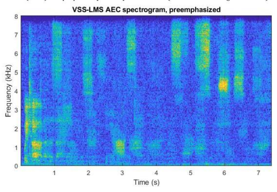
It's a different visual presentation with many signs of degradation. The messed-up adaptive tail shows that "as-is" VSS-LMS is not capable of converging above 25...30dB of ERLE (but it could be improved):
