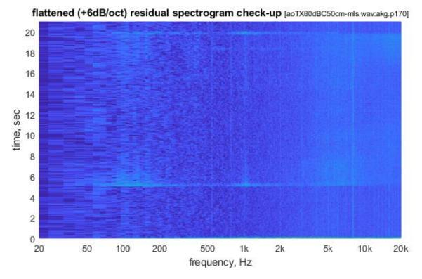
The noise-flattened spectrogram of MLS residual shows that some of the artifacts are sharp, transient, and concentrated on the excitation start/stop edges.
