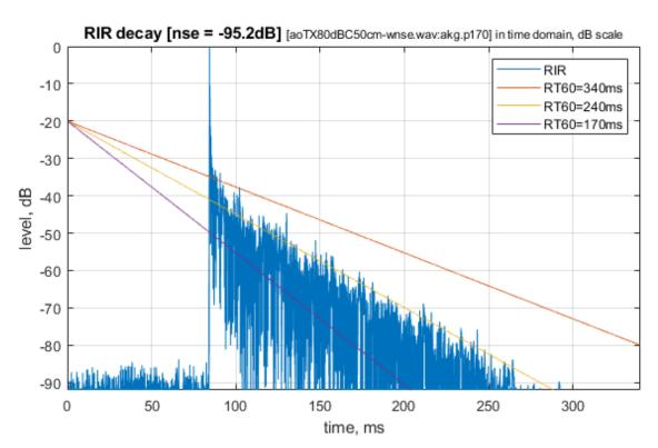
The modelling noise, besides being  $\sim$ 15 dB below MLS's, is not time-wise uniform because FSAF 'knows' that any RIR decays exponentially, and uses that to optimally bias the RIR estimate.
