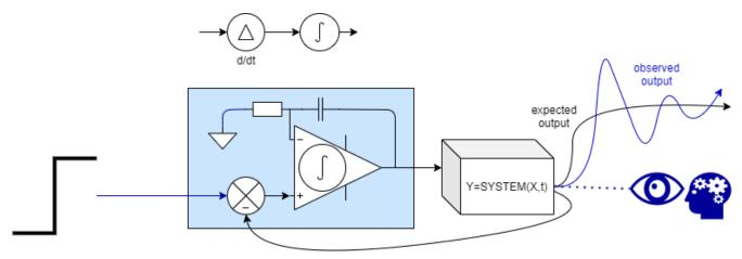
Feedback control takes frequent measurements of the system output, calculates the differences between them and the desired values (so called error signal), then integrates this differential and adjusts the system's input **X** based on the result. Instead of elaborated plans, only a general strategy is worked out prior to execution. The rest is "play by ear".
