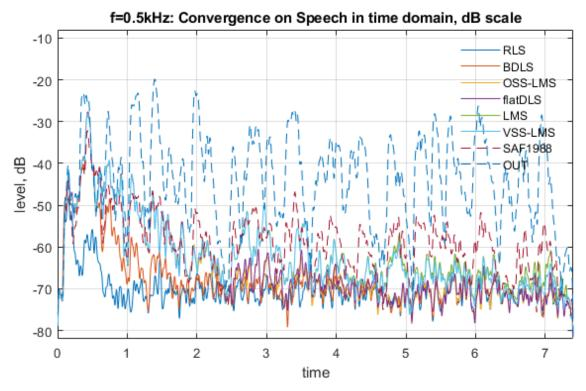
We see that SAF1988 never converges well, that either VSS-LMS or LMS converge to a degree, and the first 4 algorithms converge to the same RIR (with different the speed of convergence, of course):
