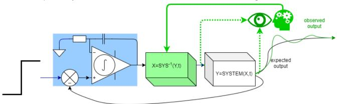
The Adaptive Control (here model-indirect, MIAC) is even less dependent on the accuracy of mathematical models of the controlled system than the Feedback Control.
