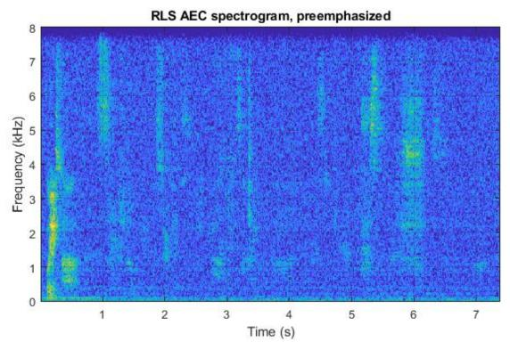
We see that RLS is able to converge perfectly within the first world, by about 0.6 seconds (for all subbands where the signal with sufficient SNR is present). The adaptive filters, with 5ms of extra delay, and 240ms of echo tail capacity, are clean:
