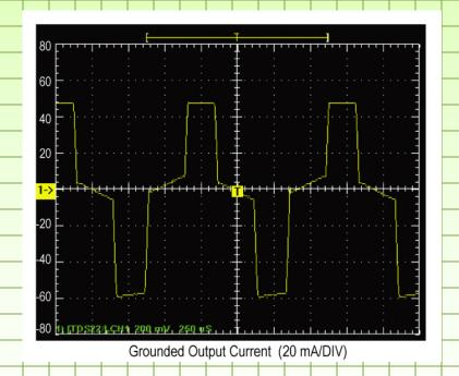
Note:  $f_{IN} = 1$  kHz,  $Z_{LOAD(+)} = 10$  k $\Omega$ ,  $Z_{LOAD(-)} = 0$   $\Omega$
