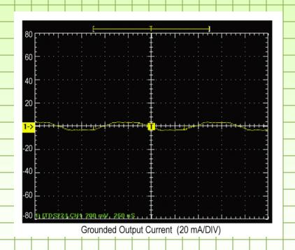
Note:  $f_{IN} = 1 \text{ kHz}$ ,  $Z_{LOAD(+)} = 10 \text{ k}\Omega$ ,  $Z_{LOAD(-)} = 0 \Omega$
