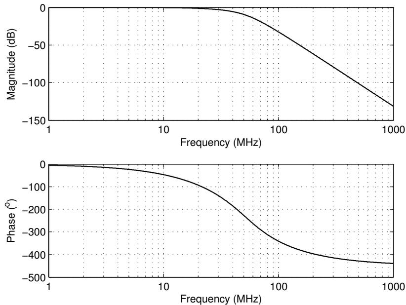
Figure 4.4: Frequency response of the DAC output filter.
