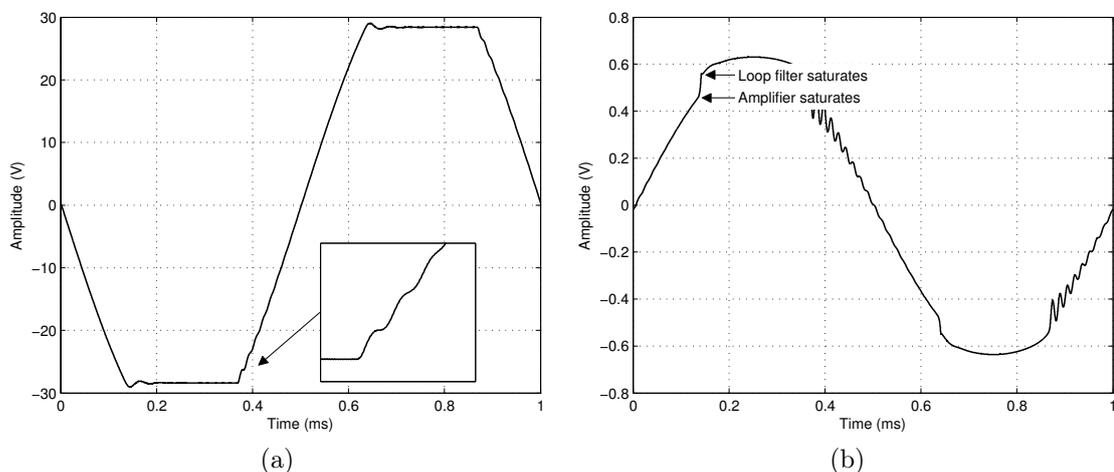
Figure 8.5: Spice simulation of amplifier output (a) and outer loop filter output (b) during over-modulation for  $R_2 = 3.3$  k $\Omega$ .
