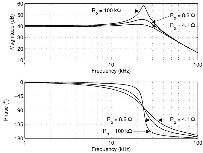
Figure 3.20: Measured open loop frequency response for various output loads. Bandwidth is  $>500\text{ kHz}$ .
