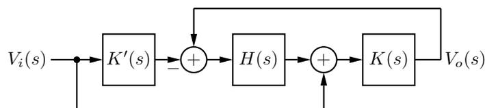
Figure 5.1: Basic control loop structure.
