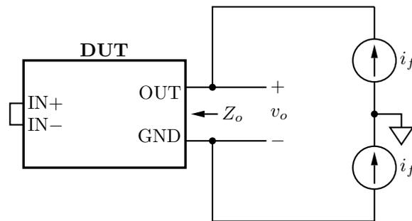
Figure 9.10: Output impedance measurement setup.
