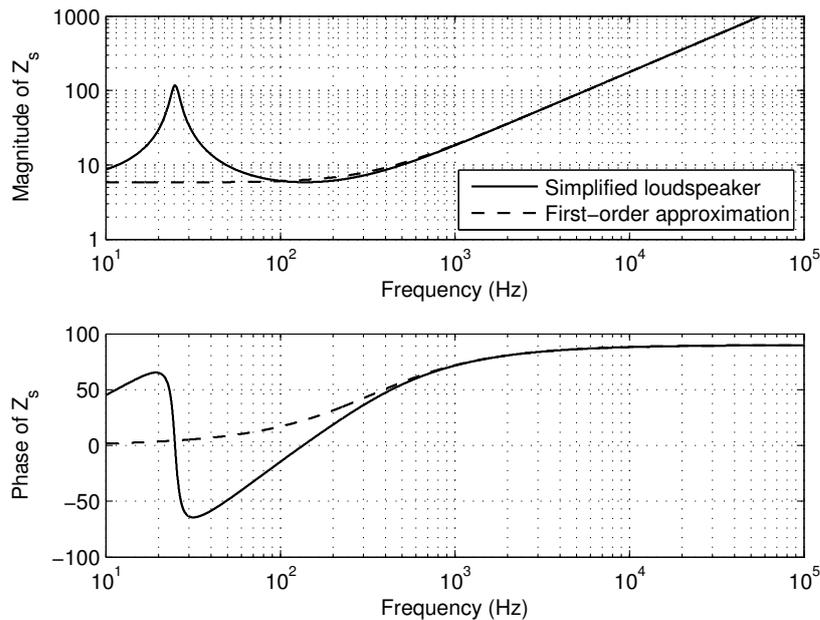
Figure 7.2: Calculated impedance of the simplified loudspeaker and the first-order approximation.
