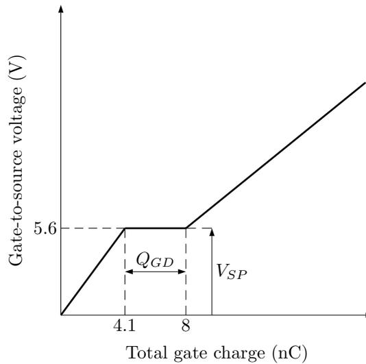
Figure 3.4: IRFI4019H-117P gate charge versus gate-to-source voltage [3].
