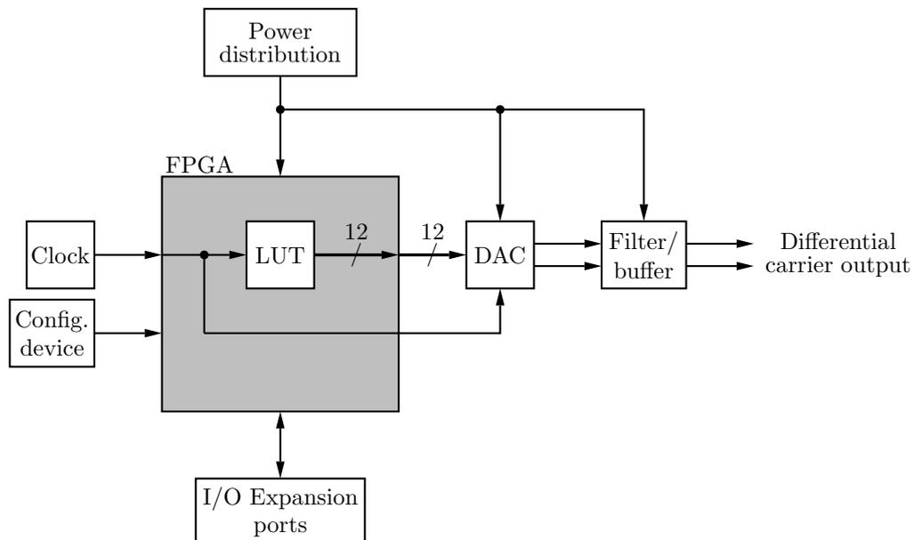
Figure 4.1: Block-diagram of the FPGA-based carrier generator.
