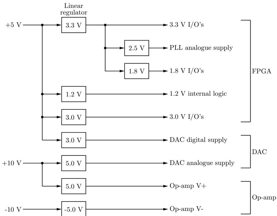
Figure 4.5: Power distribution of the carrier generator board.
