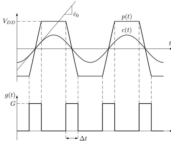
Figure 2.7: Comparator waveforms [1].
