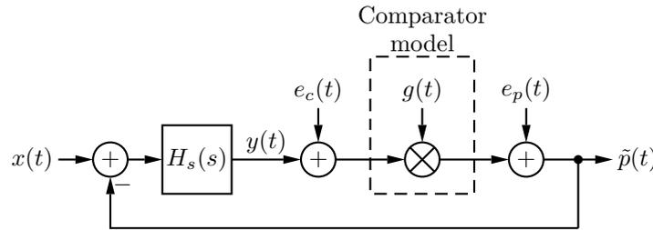
Figure 2.8: Comparator model embedded in a feedback loop.
