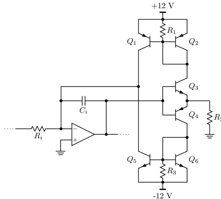
Figure 7.18: Transistor-based loop filter saturation circuit.
