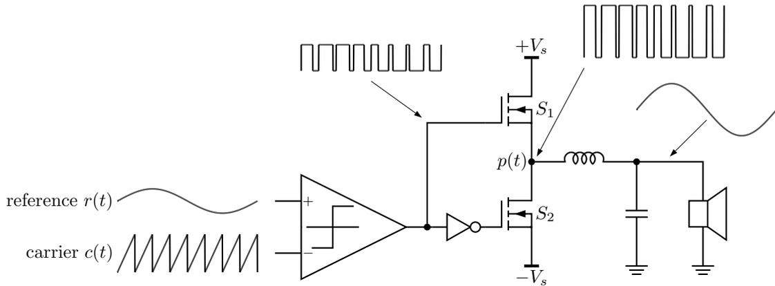
Figure 1.1: Basic class-D operation.
