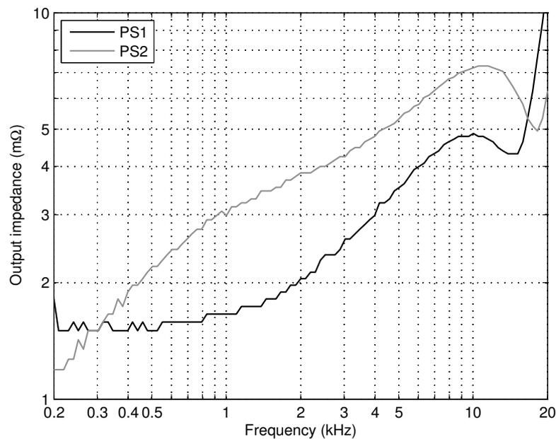
Figure 9.11: Measured output impedance for PS1 and PS2.
