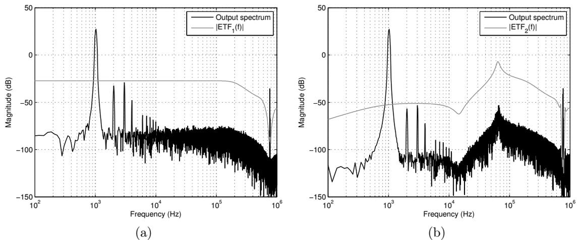
Figure 8.2: Magnitude spectrum of simulated amplifier output without ripple compensation with only the inner loop active (a) and with both loops active (b). The error transfer functions are shown in grey for comparison.
