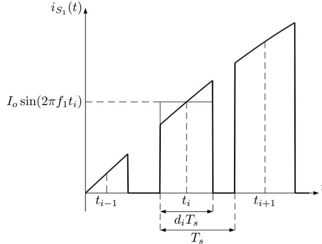
Figure 3.8: Current through MOSFET  $S_1$  with a sinusoidal current source as load. Three switching cycles are shown.
