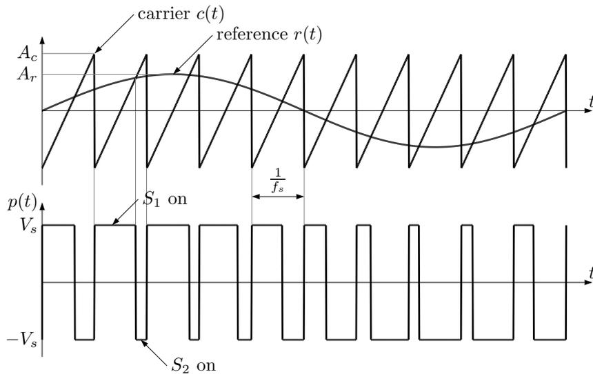
Figure 1.2: NSPWM waveforms for the converter of Figure 1.1.
