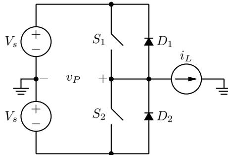
Figure 2.2: Simplified half-bridge inverter with current-source load.
