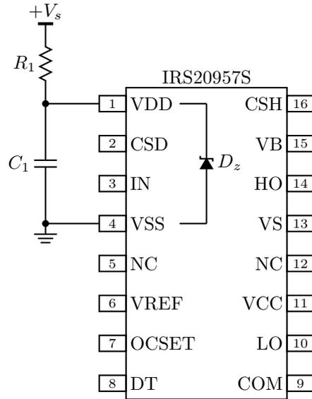
Figure 3.5: IRFI4019H-117P floating input voltage supply [3].
