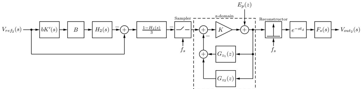
Figure 6.7: Complete loop with sampling comparator model.
