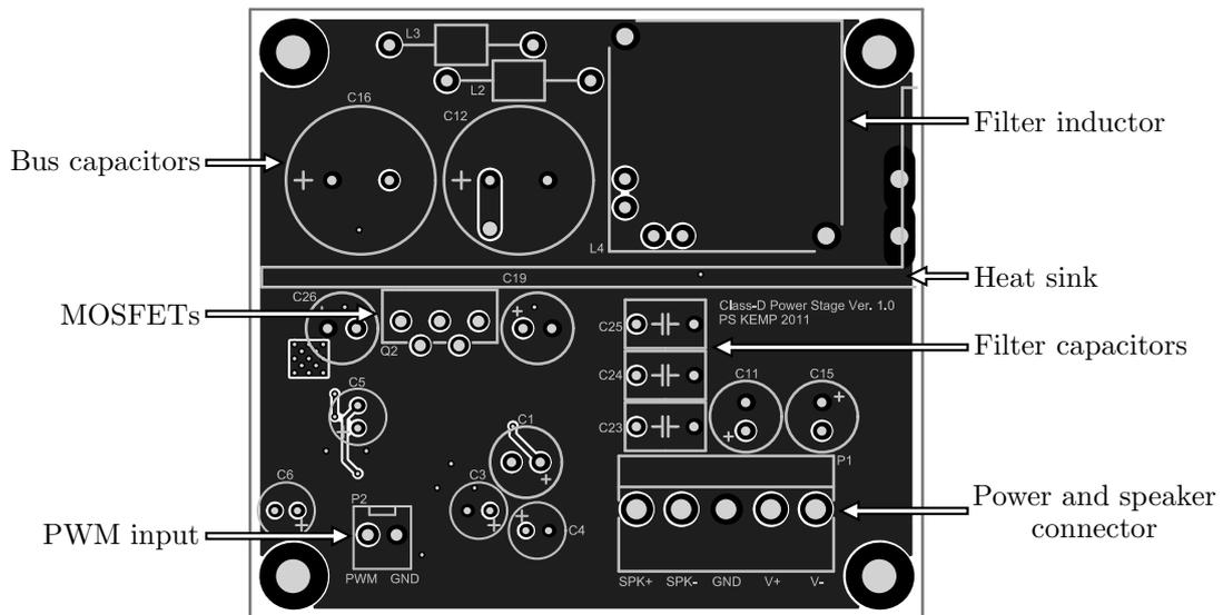
Figure 3.11: Top layer of PCB.
