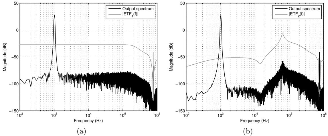
Figure 8.1: Magnitude spectrum of simulated amplifier output with only the inner loop active (a) and with both loops active (b). The error transfer functions are shown in grey for comparison.
