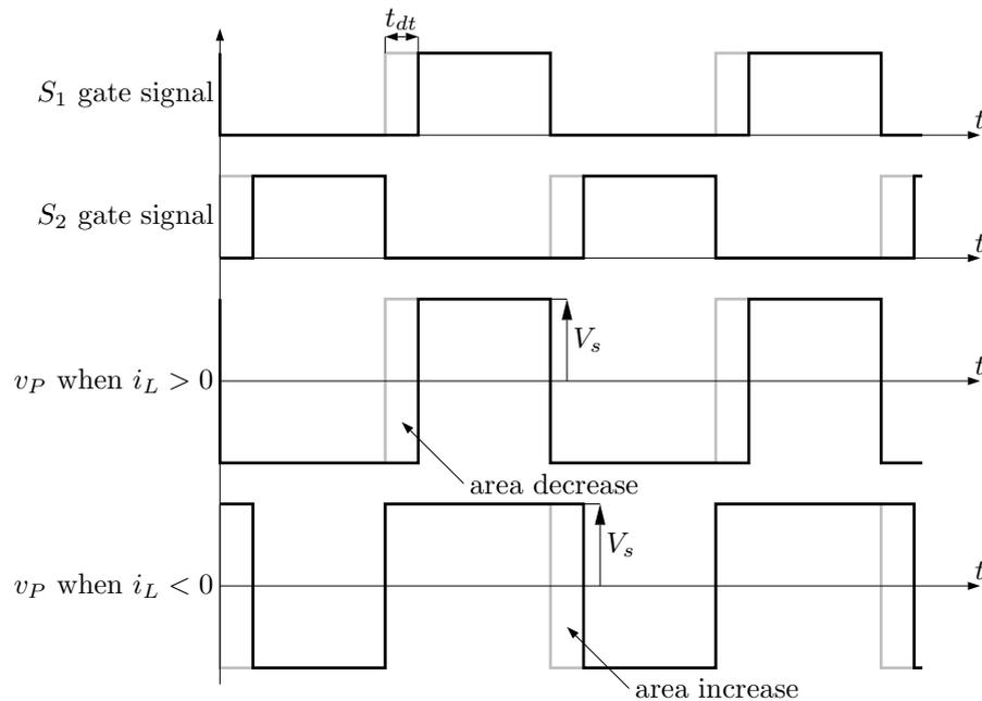
Figure 2.3: The effect of dead time on converter waveforms. Ideal waveforms are shown in grey.
