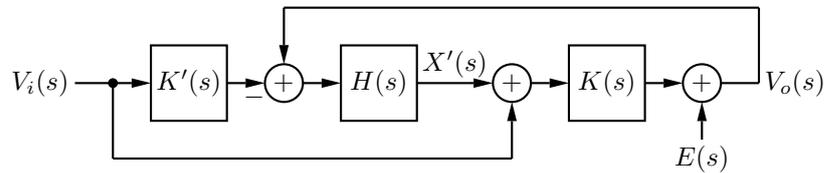
Figure 2.14: Modified control loop with deviation detection filter.
