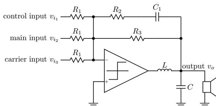
Figure 5.3: Output stage with passive lead compensation.
