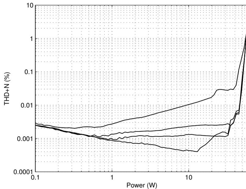
Figure 9.14: Measured THD+N versus frequency of PS1 with 1 kHz into  $8.2 \Omega$  for different values of  $t_d$ . From top to bottom: no ripple compensation,  $t_d = 175$  ns,  $t_d = 150$  ns, and  $t_d = 125$  ns.
