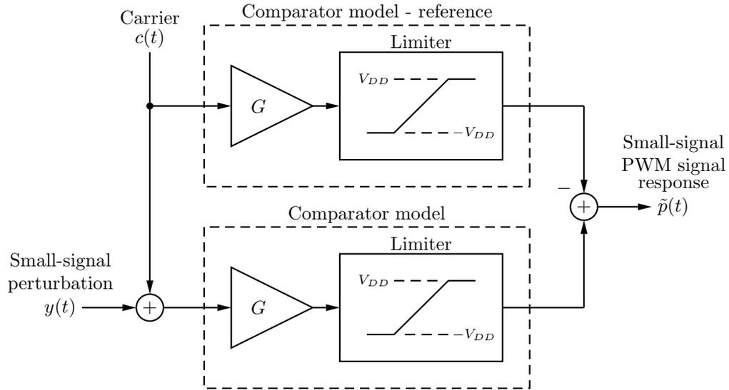
Figure 2.6: Small-signal comparator model [1].
