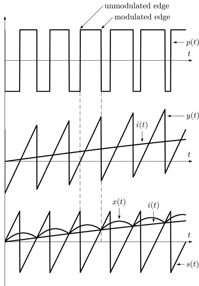
Figure 2.11: Ripple compensation waveforms for a first-order loop [2].
