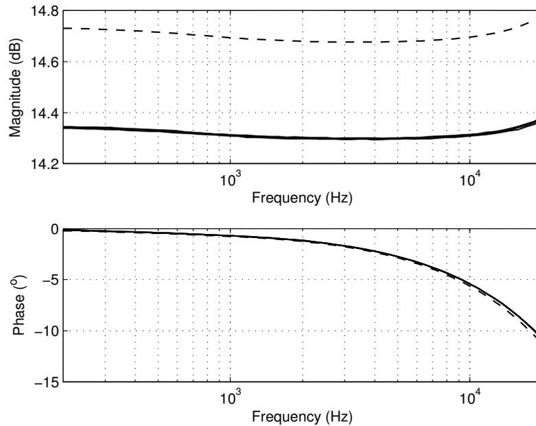
Figure 9.9: Measured closed loop frequency response of the complete control loop for various output loads. From top to bottom:  $R_o = 100 \text{ k}\Omega$ ,  $R_o = 8.2 \Omega$  and  $R_o = 4.1 \Omega$ . The dashed line is the theoretical frequency response for an  $8.2 \Omega$  load.
