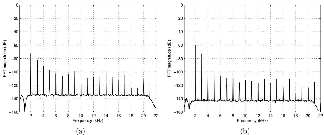
Figure 9.5: FFT of the distortion residue with the inner loop active with 10 W at 1 kHz into  $8.2 \Omega$  for (a) PS1 and (b) PS2. THD+N is (a) 0.0254% and (b) 0.0985%. The suppressed fundamental is at 0 dB.
