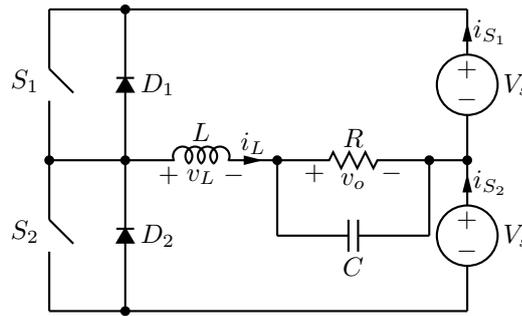
Figure 2.4: Simplified half-bridge converter.
