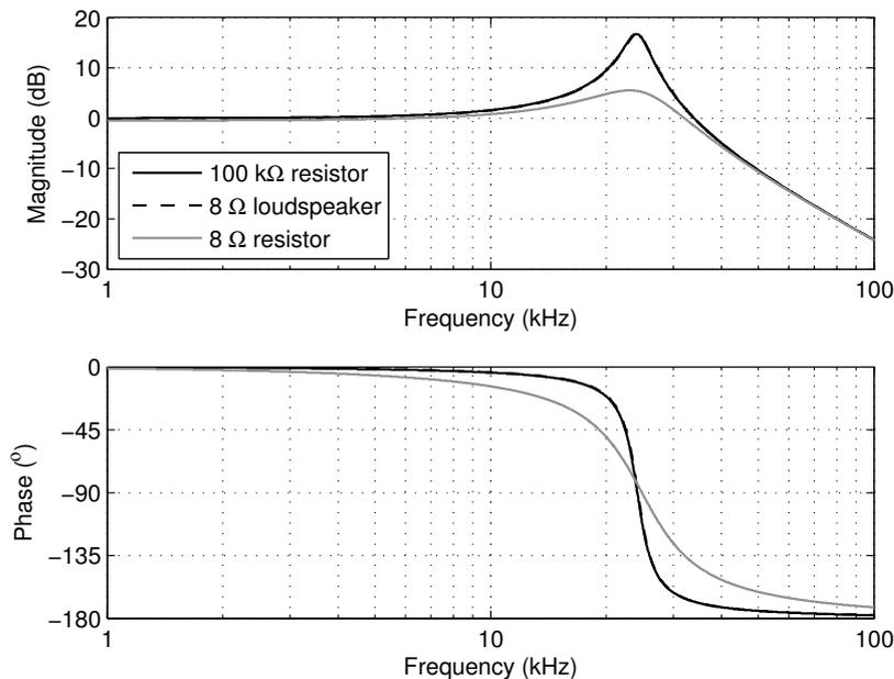
Figure 7.3: Calculated demodulation filter transfer function for a  $100\text{ k}\Omega$  resistor, an  $8\ \Omega$  loudspeaker, and an  $8\ \Omega$  resistor as load, respectively.
