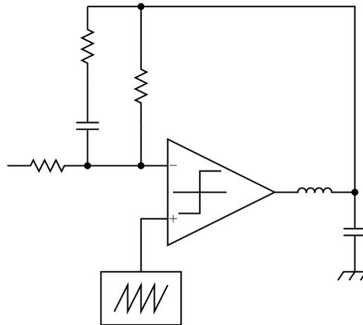
Figure 2.15: Output stage with passive lead network.
