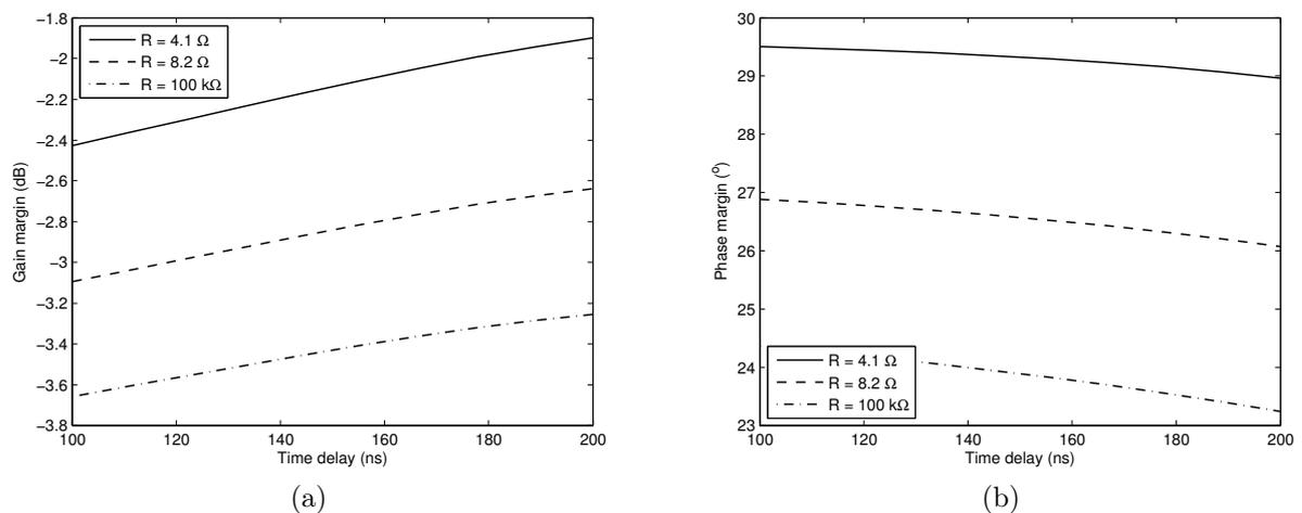
Figure 7.13: Gain margin (a), and phase margin (b), versus propagation delay for different loads.
