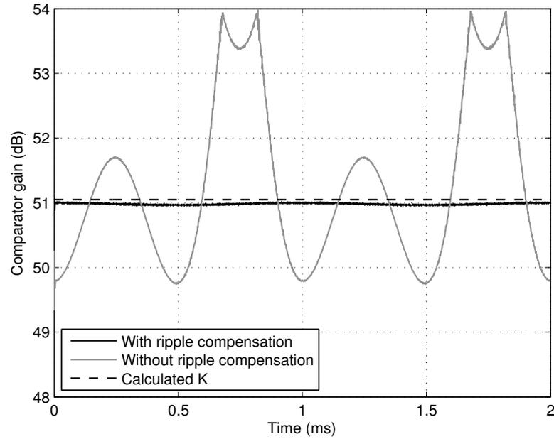
Figure 8.3: Simulated comparator gain with and without ripple compensation. The input signal frequency is 1 kHz and  $m_a = 0.8$ .
