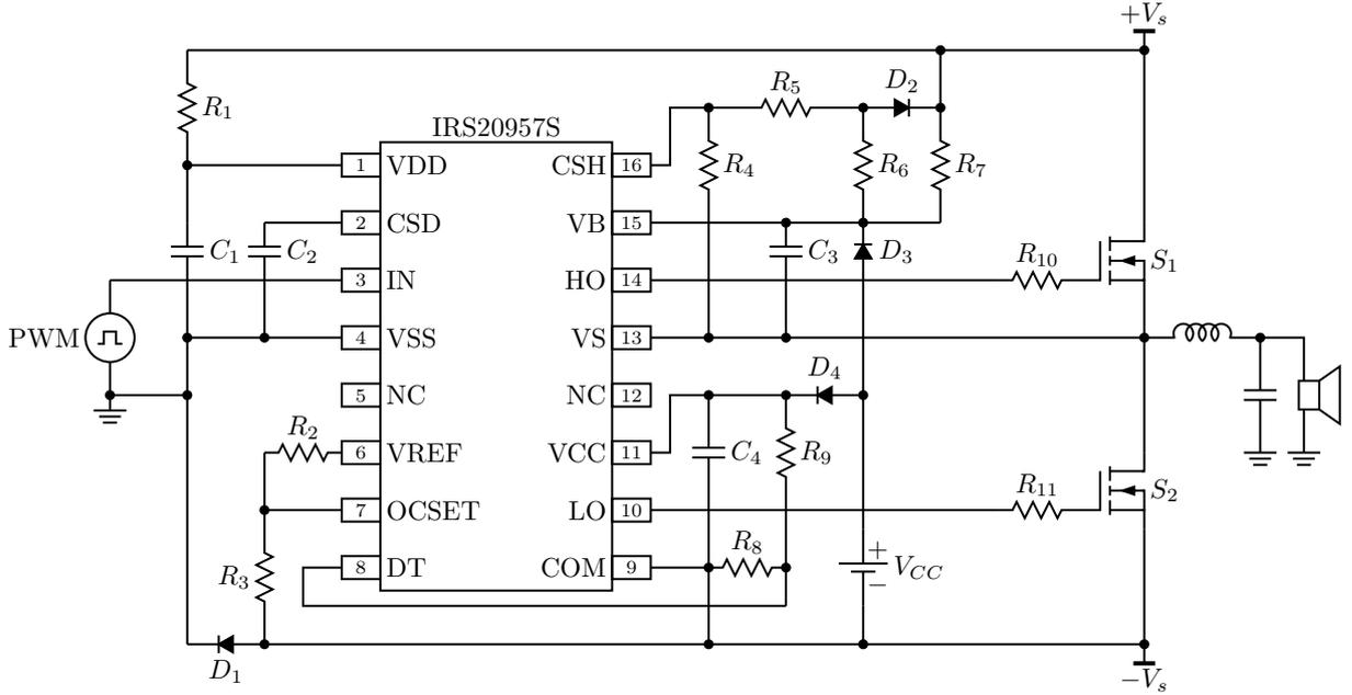
Figure 3.2: IRS20957S gate driver implementation.
