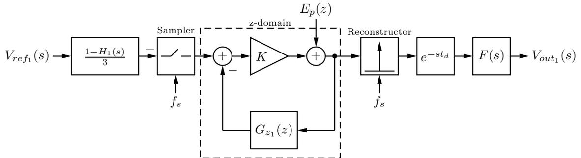
Figure 6.5: Inner loop with sampling comparator model.
