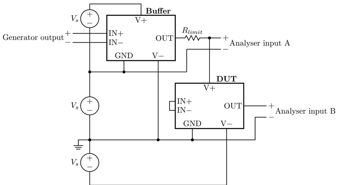
Figure 9.12: PSRR measurement setup.
