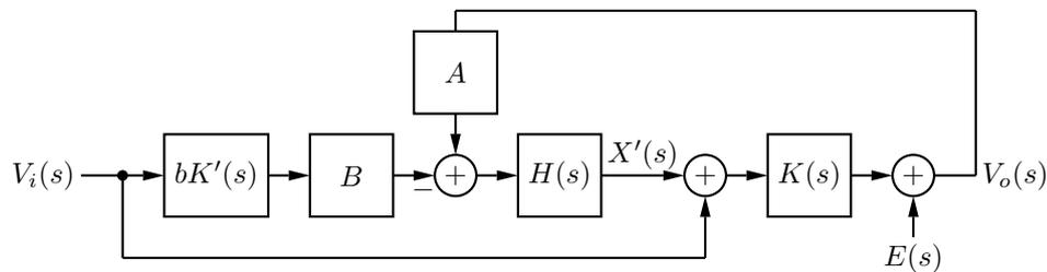
Figure 7.8: General control system with estimation filter.
