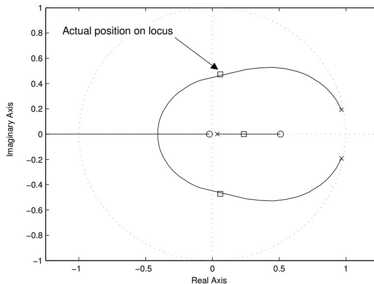
Figure 7.9: Root locus of the inner control loop with an output load of  $R_o = 100 \text{ k}\Omega$ .
