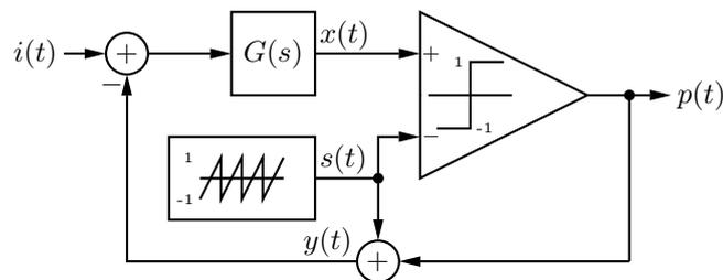
Figure 2.10: Simple PWM feedback loop with ripple compensation [2].
