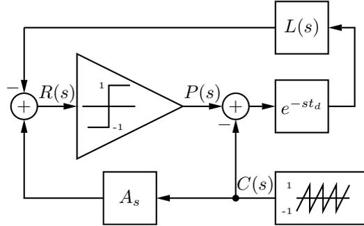
Figure 6.3: Block diagram for comparator gain calculation.
