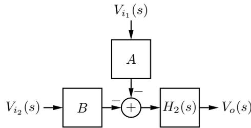
Figure 5.7: Control system block diagram of single op-amp third-order integrating loop filter.
