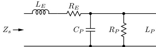
Figure 7.1: Simplified equivalent circuit of a moving-coil transducer.
