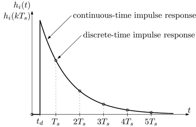
Figure 6.2: Continuous-time and discrete-time impulse responses.
