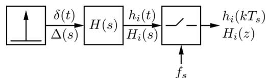
Figure 6.1: Block diagram illustration of the impulse invariant method.
