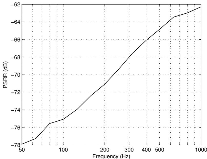
Figure 9.13: Measured PSRR as a function of frequency.
