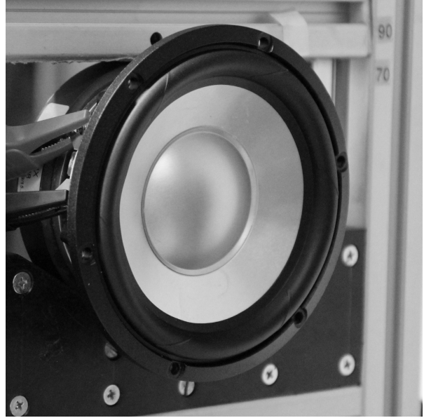
Fig. 1. SEAS L16RNX (H1488-08) mid-woofer mounted in stand.
