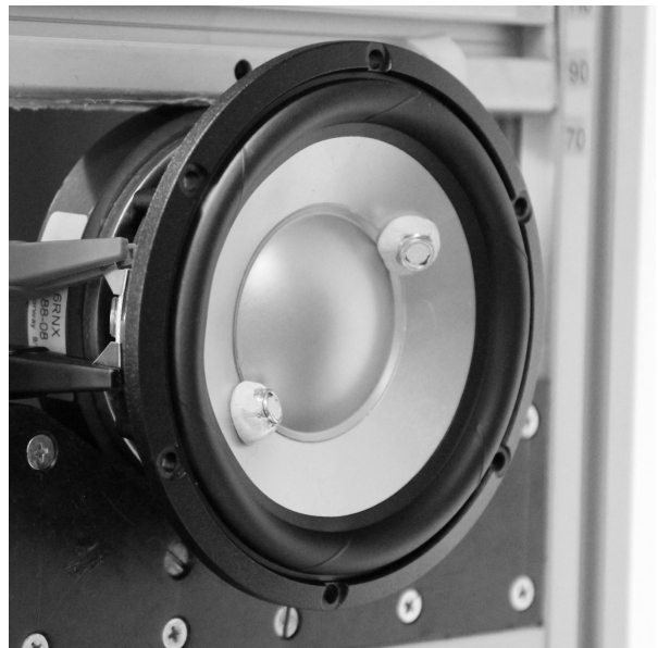
Fig. 2. SEAS L16RNX (H1488-08) mid-woofer mounted in stand with added mass m_1 .
