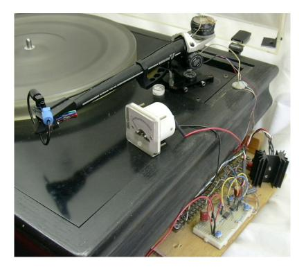
**Warps**: Additionally, I expected such a sensor control circuit could (in theory) be tuned to track record warps even better than the passive magnets version, by both following warps in real time, and by damping any resultant resonance in the arm levitation magnets, and in turn perhaps also damping cartridge and turntable suspension resonances. However, active feedback yielded little if any improvements in these areas compared to the already very good passive electromagnet version.
