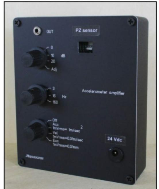
Photo 2: For the completed amplifier. I used the same metal box from Hammond and the aluminum frontplate that I had designed for the ACH-01 amplifier.
