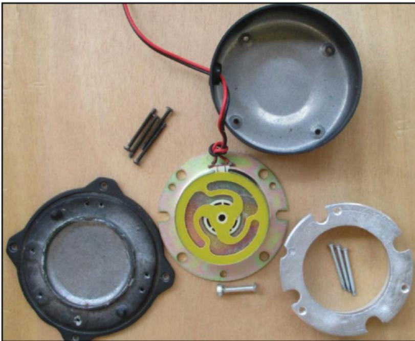
Photo 3: The disassembled Visaton BS-130 unit
