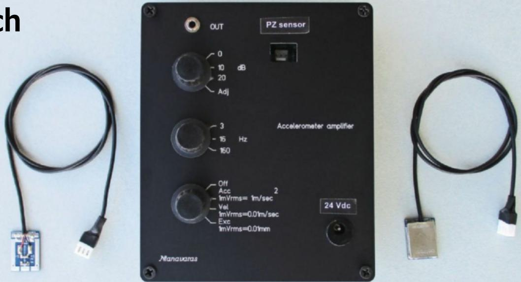
Several years ago, George Ntanavaras designed a system consisting of the ACH-01 accelerometer and an amplifier with an integrated analog signal processor. Over the years, he has been looking for other possible solutions concerning the vibration measurements. In this article, he describes his research for the design, the construction of such a system, and presents the results and the measurements.
