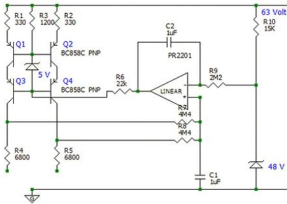
Figure 2. Current-source design – True Phantom.
