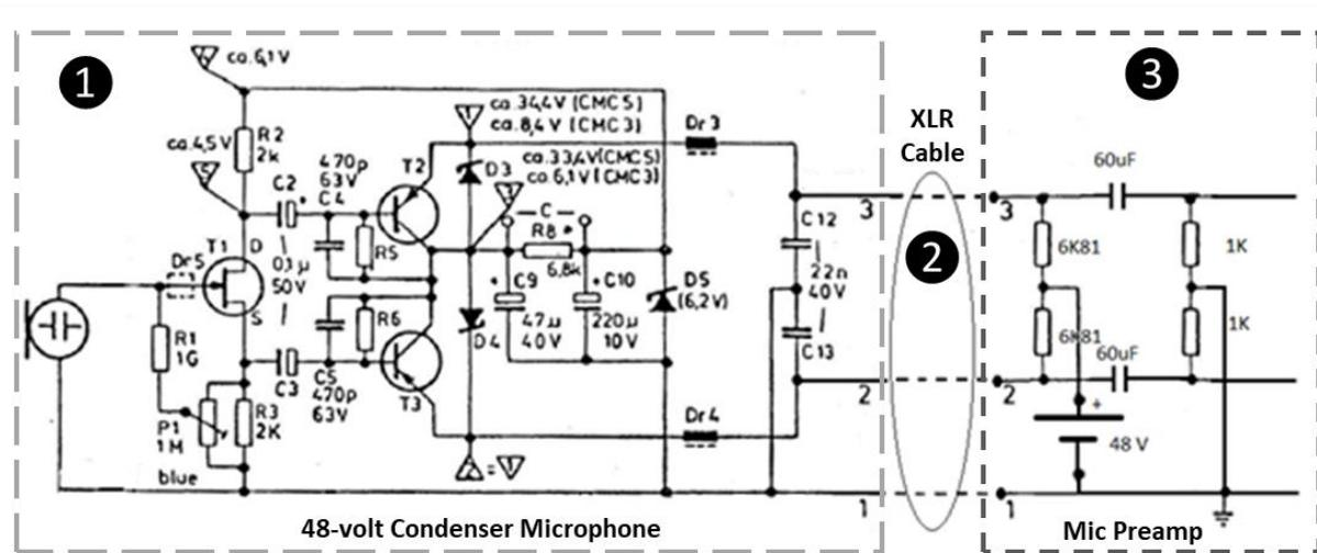
Figure 1. Complete microphone system.
