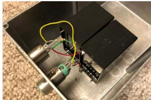
Figure 6. Metal box with DC-blocking
