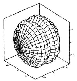
Figure 18 3D polar response (smoothed) of 0.3 m^2 DML panel, 8kHz
