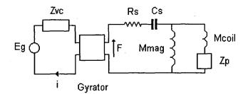
Figure 9 Complete electromechanical schematic for a DML panel and exciter
