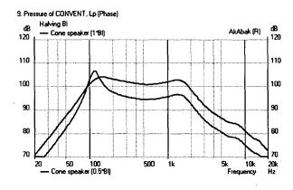
Figure 11 Traditional moving coil loudspeaker SPL, when BI factor is halved
