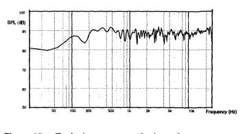
Figure 15 Typical unsmoothed frequency response of a DML panel
