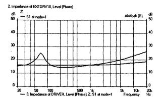
Figure 13 Comparison of Traditional loudspeaker terminal impedance, versus DML panel
