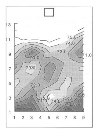
Figure 19 Room pressure contours from traditional loudspeaker, positioned at front centre
