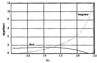
Figure 10 Typical panel impedance presented to the driving point
