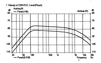
Figure 12 DML loudspeaker mean panel velocity, when BI factor is halved
