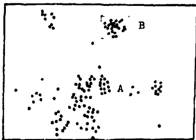
Fig.1 A part of the f-autoradiogram of distribution of U in Al (100x)
