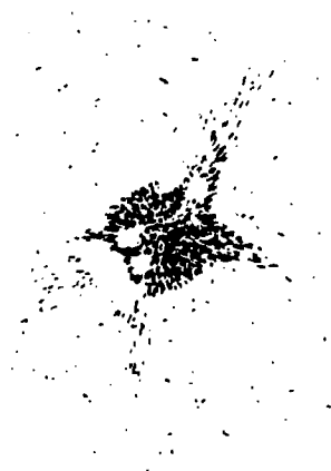
Figure 4. A characteristic distribution of uranium and plutonium in the 'hot particles' found in the soils of Chernobyl zone
