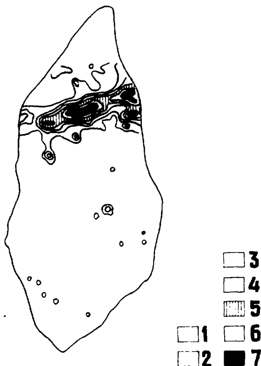
Figure 4. Gold distribution concentration profiles obtained by photometering a quartz section over 0.15 \text{ mm}^2 square (the gold content is given): 1 - less than 1 \cdot 10^{-6} \text{ g} , 2 - (1+2.6) \cdot 10^{-6} \text{ g} , 3 - (2.6+4.6) \cdot 10^{-6} \text{ g} , 4 - (4.6+7.5) \cdot 10^{-6} \text{ g} , 5 - (7.5+11.0) \cdot 10^{-6} \text{ g} , 6 - (11.0+16.6) \cdot 10^{-6} \text{ g} , 7 - (16.6+25.1) \cdot 10^{-6} \text{ g}
