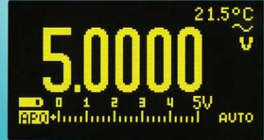
Large numerical display that's toggleable to dual display mode, both at 50,000-count high resolution
