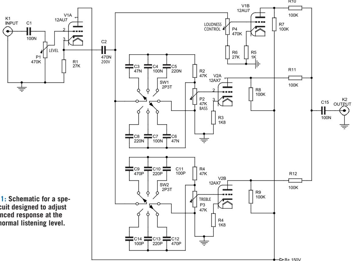
**FIGURE 1:** Schematic for a special circuit designed to adjust for balanced response at the lowest normal listening level.
