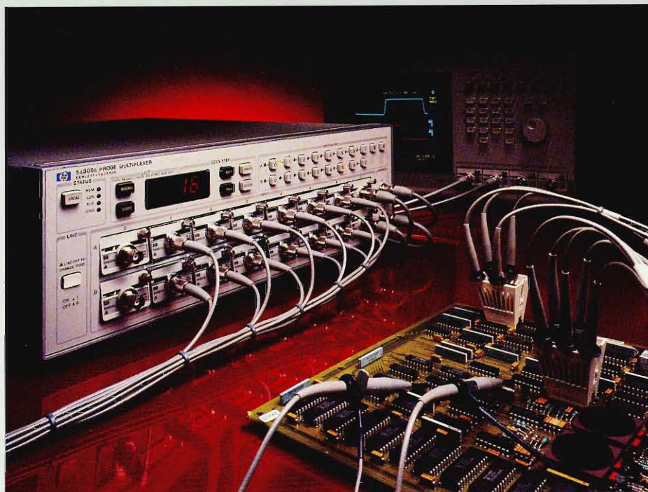
The HP 54300A probe multiplexer expands the input capability of the HP 54100 and HP 54110 digitizing oscilloscopes, or any 50Ω input instrument, simplifying delicate high-frequency connections.
