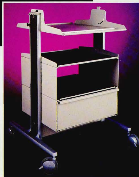
HP 1008A opt 006: Storage cabinet with shelf on top and drawer in lower position; load limit 18 kg (40 lb) each on shelf and in cabinet, 11 kg (25 lb) in drawer.
