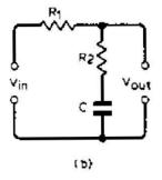
Flg.7. Transitional lag circuits. Both circuits are equivalent and give no phase lag at zero or infinite frequencies, but contribute a phase lag which reaches a maximum value at the geometric mean of the two 'corner' frequencies. See text.
