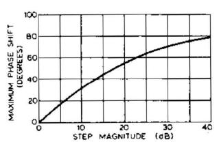
Fig. 8. Characteristic for simple transitional lag or lead circuits.
