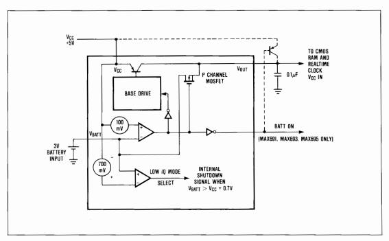
Figure 4. Battery-Switchover Block Diagram
