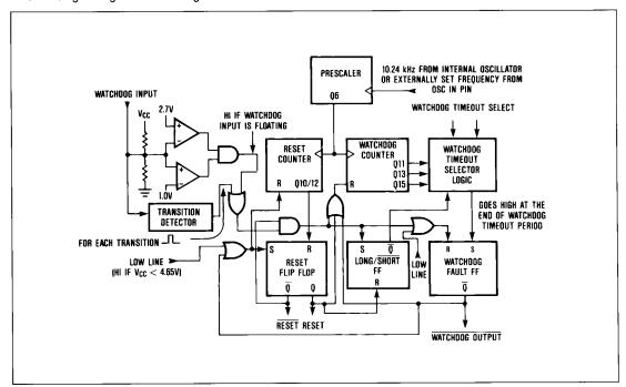
Figure 7. Watchdog Timer Block Diagram
