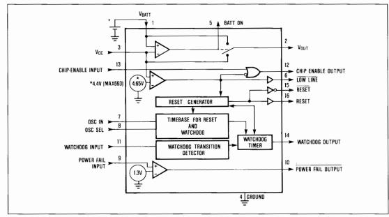
Figure 3. MAX691/693/695 Block Diagram
