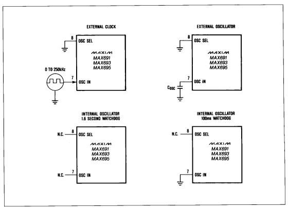
Figure 8. Oscillator Circuits
