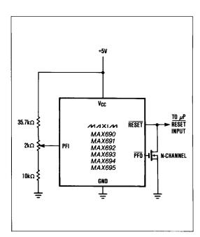
Figure 10. Reset on Overvoltage or Undervoltage
