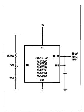
Figure 9. Externally Adjustable V<sub>CC</sub> Reset Threshold
