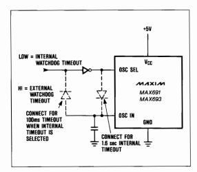
Figure 14. Selecting Internal or External Watchdog Timeout
