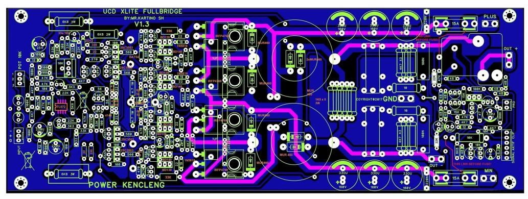
Note: TL072 installed to be upside down at bottom
