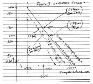
The LOWER dashed line is the line for a bias of 1 uA. It has a slope of -2.200 mV/degree C. It's offset by 60 mV/decade at room temperature, more when hot, and less when cold. The tiny segment of the line is at 0.1 uA, and has a slope of -2.400 mV/degree C (Fig. 3).
