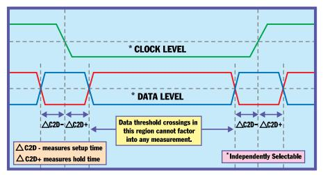
Setup and Hold Time Parameter Diagram
