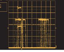
Above, Exclusion Trigger is set to eliminate pulses within a width of 50 ns. Only pulse widths that are not 50 ns wide will trigger the scope.
