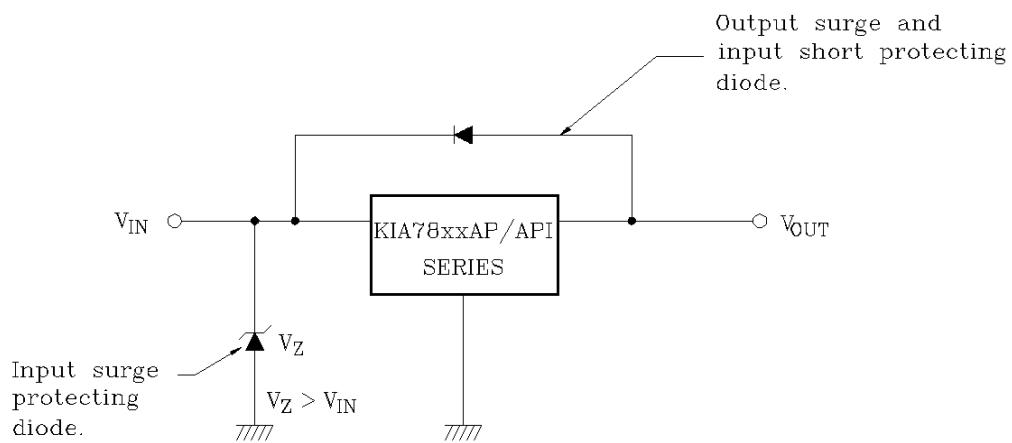
(3) When the input voltage is too high, the power dissipation of three terminal regulator increase because of series regulator, so that the junction temperature rises.
