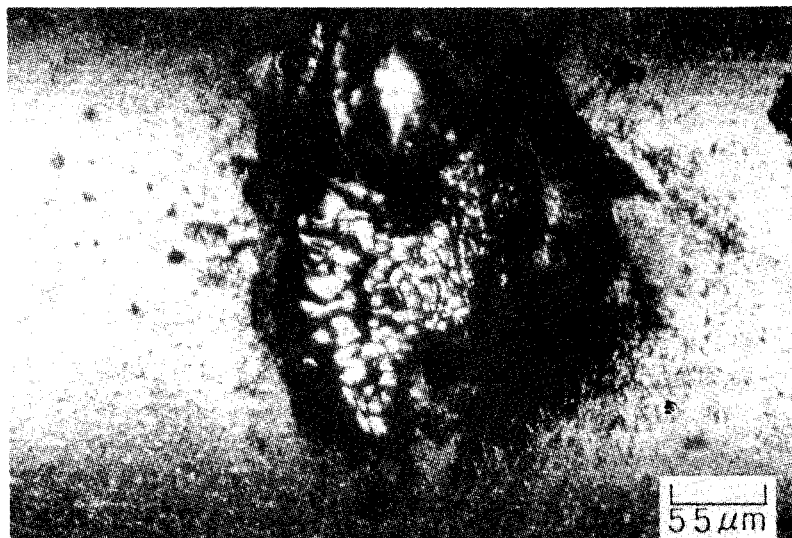
Contact Surfaces After 18-VDC, 45-mA Load Test
