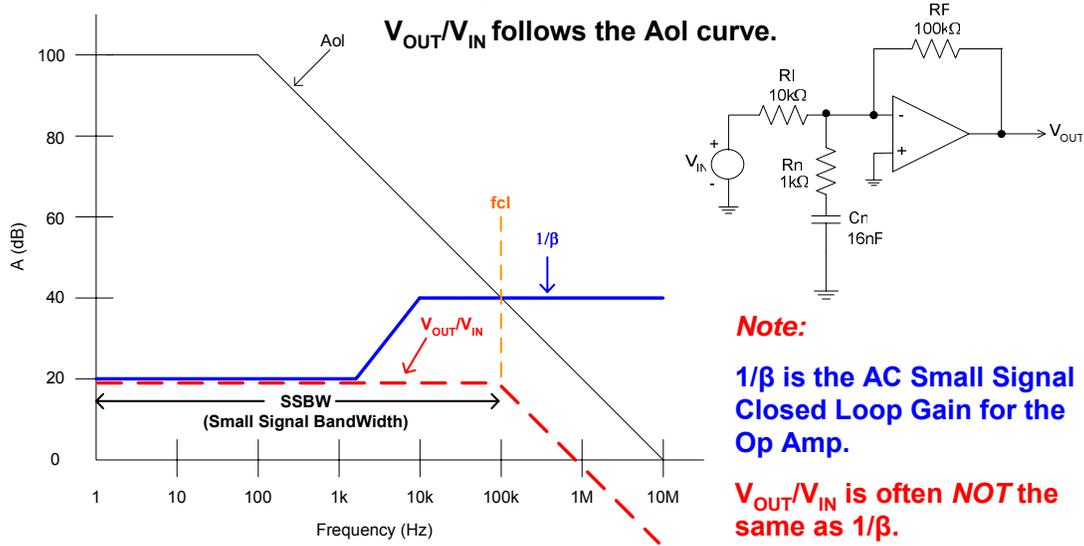
**Fig. 1.23:  $V_{OUT}/V_{IN}$  Vs  $1/\beta$**
