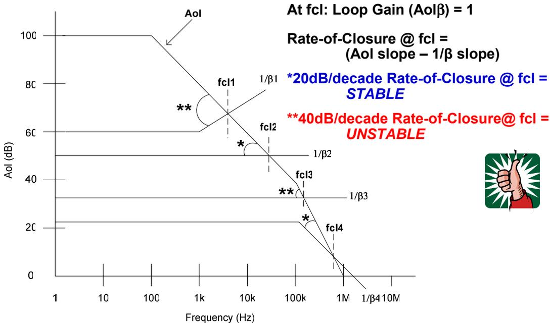
**Fig. 1.20: Rate-Of-Closure Test for Loop Gain Stability**
