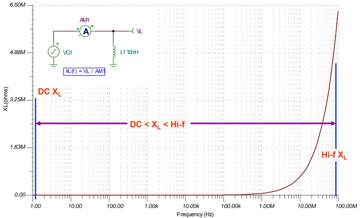
Fig. 1.13: Intuitive Inductor Model SPICE Simulation
