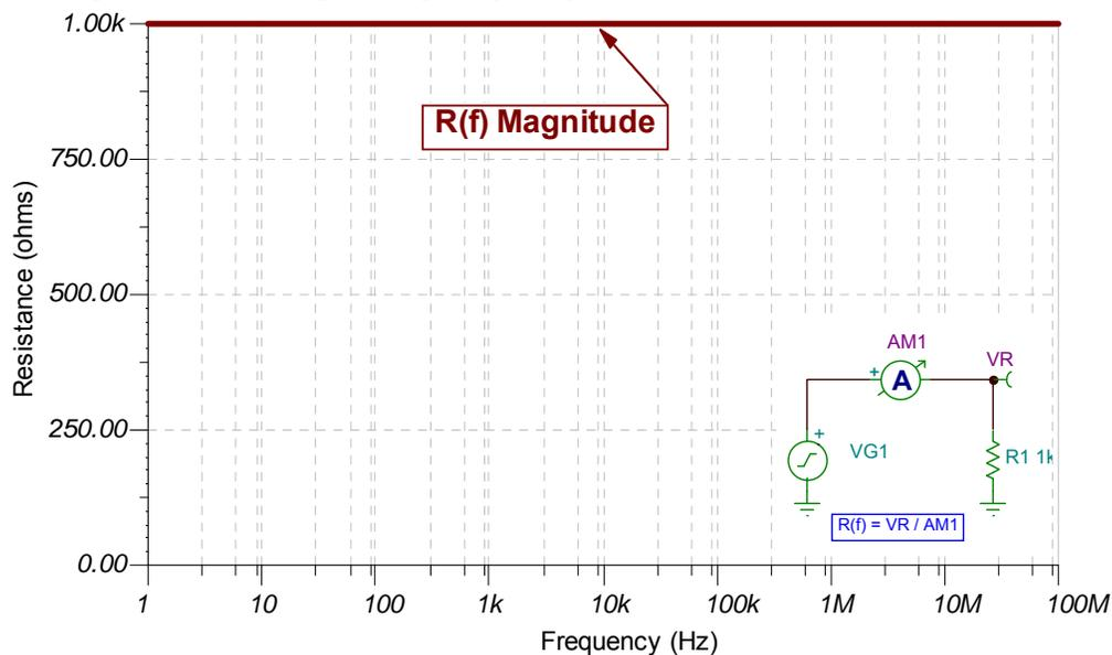
**Fig. 1.9: Intuitive Resistor Model**
