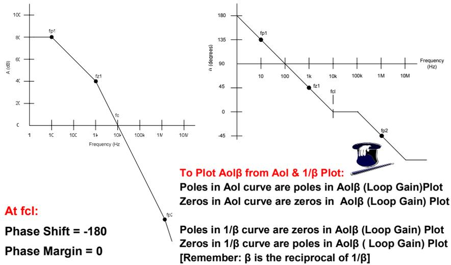
**Fig. 1.22: Loop Gain Plot From Aol Curve &  $1/\beta$  Plot**
