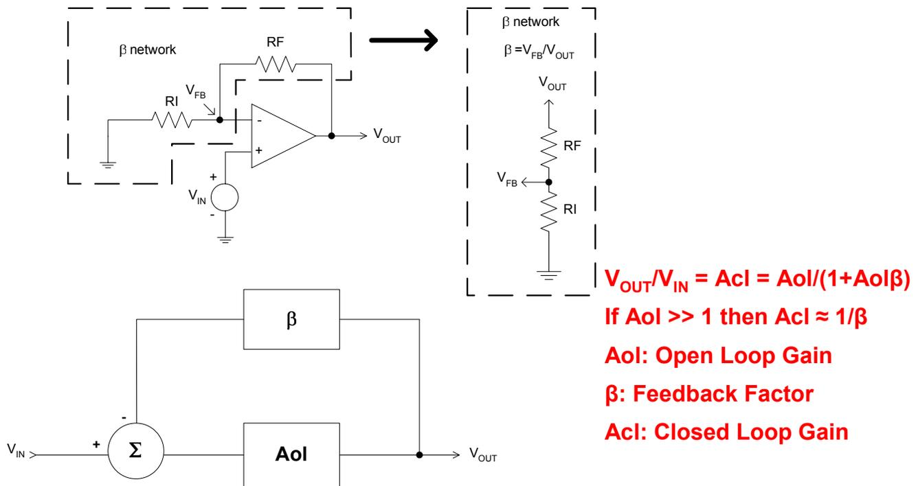
Fig. 1.14: Op amp Loop-Gain Model
