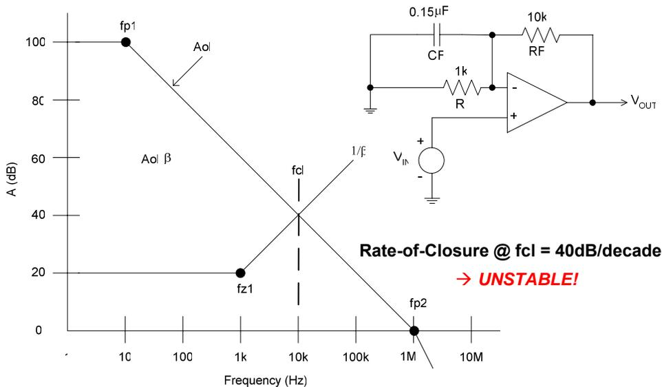
**Fig. 1.21: Loop Gain Stability Example**
