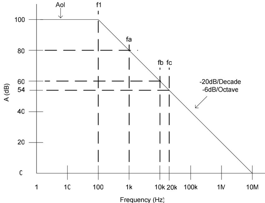
**Fig. 1.4: Magnitude Bode Plot: 20 dB/Decade = 6 dB/Octave**
