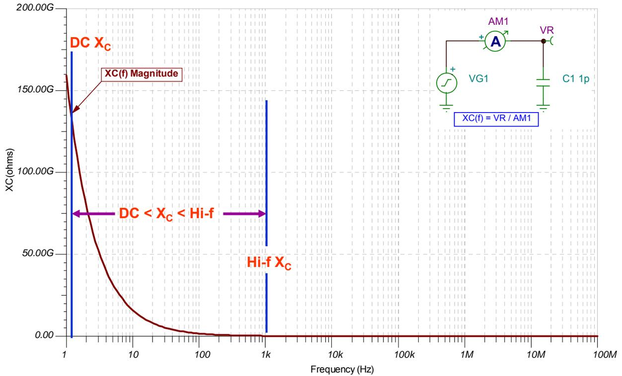
Fig. 1.11: Intuitive Capacitor Model SPICE Simulation
