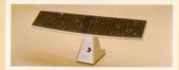
SH-F101 A compact indoor antenna that dramatically improves reception in strong signal areas. Within the 43cm wide antenna is a zig-zag pattern antenna element and two varactor diodes and coils to provide internal electronic tuning.
