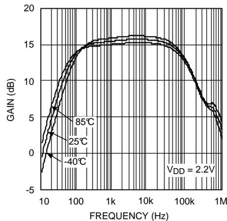
Figure 25. LMV1012-15 Gain vs. Frequency Over Temperature
