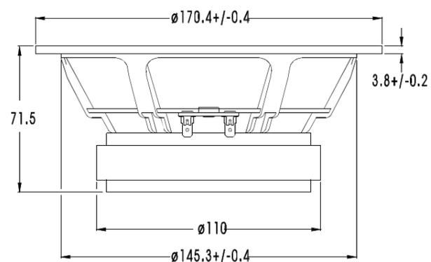
P17REX is a 6,5" High Fidelity woofer with an injection moulded metal chassis. A polypropylene based cone, a soft PVC dust cap and a high loss rubber surround are carefully matched to each other, resulting in an outstandingly smooth frequency response. The unit has a high power handling capacity due to its relatively large voice coil diameter. The magnet system has a T-shaped cross section of the pole piece for low modulation distortion. A large magnet system provides high efficiency and low Q.
