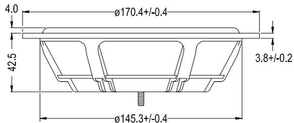
SP17R is a 17cm (6,5") passive radiator intended for use, as an alternative to the vented port in a bass reflex cabinet, together with an active woofer of similar size or smaller.
