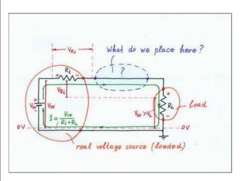
If we load a real voltage source having internal resistance, it droops.
