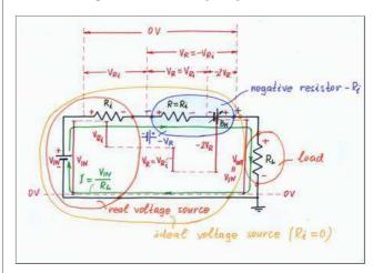
**Recipe:** In order to compensate a "positive" resistor R, add in series a negative resistor -R.
