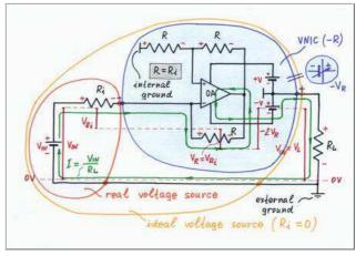
In an NIC, the op-amp acts just as a small battery, which adds so much voltage as it loses across the resistor Ri.
