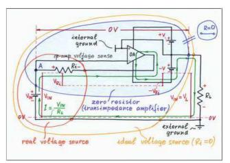
A transimpedance amplifier is another circuit, which can compensate resistive losses by means of negative feedback. It is precise and economical circuit; only, it needs an additional voltage sense wire.
