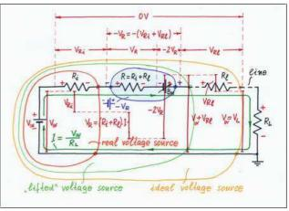
A negative resistor -(Ri + R<sub>I</sub>) neutralizes the "positive" resistance (Ri + R<sub>I</sub>).
