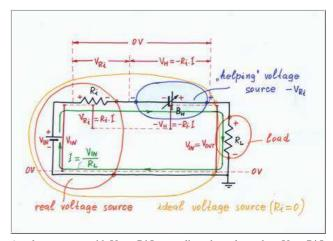
A voltage source with  $V_{\text{H}}\!=$  -Ri.I neutralizes the voltage drop  $V_{\text{Ri}}\!=$  Ri.I.
