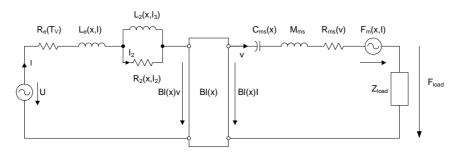
The lumped-parameter model shown above is used to describe the large signal behavior of electro-dynamical drivers at high amplitudes. In contrast to the well known linear model the elements
