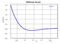
The stiffness  $K_{ms}(x)$  which is the inverse of the compliance  $C_{ms}(x)$  describes the ratio of the instantaneous force and displacement at the working point x. A high increase of the stiffness indicates the limit of the moving capability of the mechanical suspension. Variation of  $K_{ms}(x)$  corresponds with instantaneous variation of the resonance frequency  $f_S(x)$  and the mechanical loss factor  $Q_{ms}(x)$  versus displacement.
