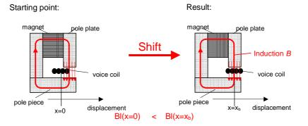
DC offset generated by asymmetrical port geometry An asymmetrical shape of the port may cause a rectification of the air flow in vented enclosures. The generation of a pressure difference at the port's orifices may generate a significant dynamic shift of the rest position of the coil.
