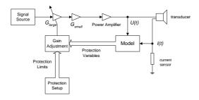
The measurement of the large signal parameters starts in the small signal domain and performs a slow increase of the signal amplitude (enlargement mode) up to the thermal and mechanical limits of the transducer. To avoid an overload or damage a protection system determines the maximal signal amplitude admissible for the particular driver and limits the excitation signal when protection variables (such as voice coil temperature, BI or compliance variation) exceed user defined limit values.
