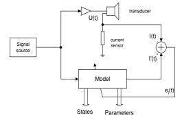
The transducer model is implemented as an adaptive system in a digital signal processor (DSP). The transducer is persistently excited by an audio-like signal generated by a signal source via a power amplifier. The model excited with the voltage U(t) estimates the voice coil current I(t)' and compares with the measured current I(t). The amplitude of the difference signal (error) is minimized by adjusting the model parameters adaptively. The output parameters
