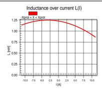
The nonlinear B(H) characteristic of the iron causes a variation of the inductance L(i) versus voice coil current i. This nonlinearity is also called flux modulation or better permeability modulation. An symmetric characteristic shows a saturation of the iron at high positive and negative current. The curve becomes asymmetric for a high DC flux generated by the magnet. The parameter L(i) causes harmonic distortion at higher frequencies which can easily be detected in the input current.
