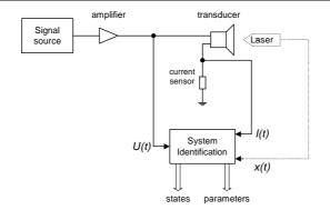
An inexpensive laser sensor based on triangulation principle (see A2 Laser Displacement Sensor) can be used for measuring the voice coil displacement during the test. This information is used to calibrate the mechanical parameters in absolute terms.
