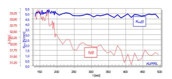
The properties of the mechanical suspension vary with time due to reversible and nonreversible processes (creep, ageing).
