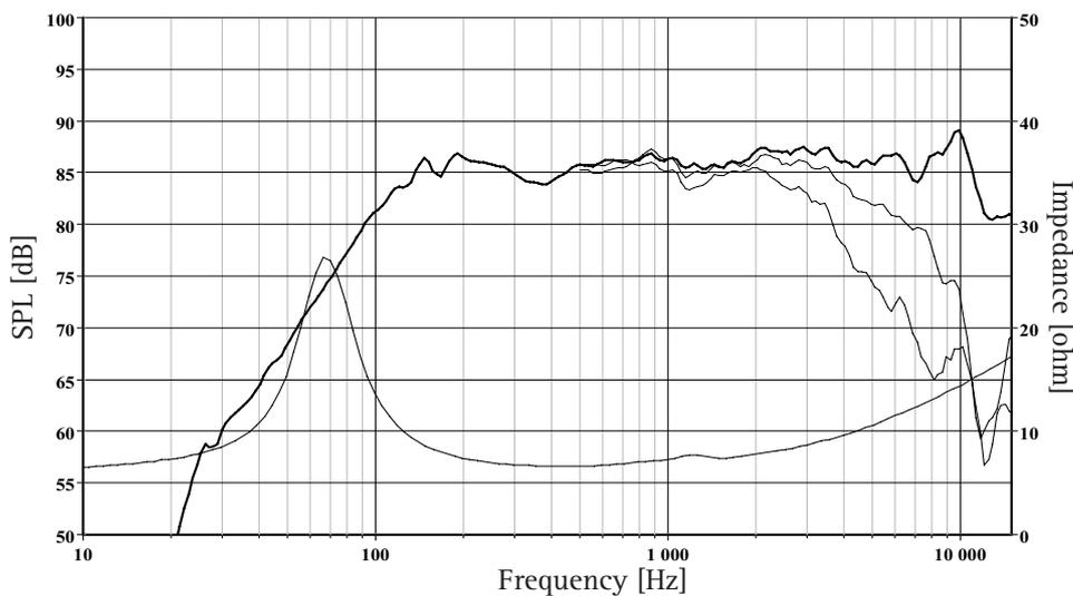
The frequency responses above show measured free field sound pressure in 0, 30, and 60 degrees angle using a 0.8L rear chamber mounted in a standard IEC baffle. Input 2.83 V<sub>RMS</sub>, microphone distance 0.5m, normalized to SPL 1m. The impedance is measured in free air without baffle using a 2V sine signal.
