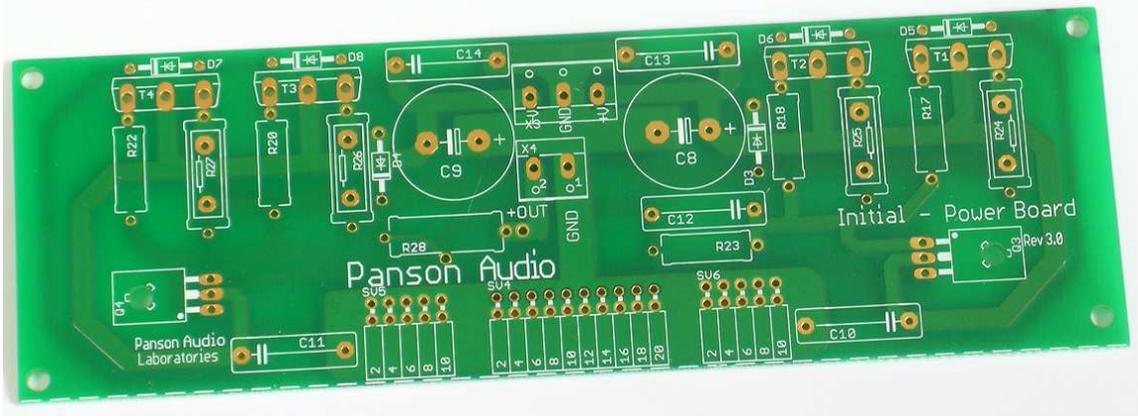
Figure 5 Power board for 3-Lead TO-264 packaged output transistors.
