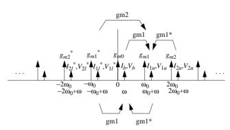
Time-varying conductances and capacitances are expanded into Fourier coefficients. Noise voltages at different sidebands can be obtained by convolving the noise current spectrum i with the line spectrum of the nonlinear components:
