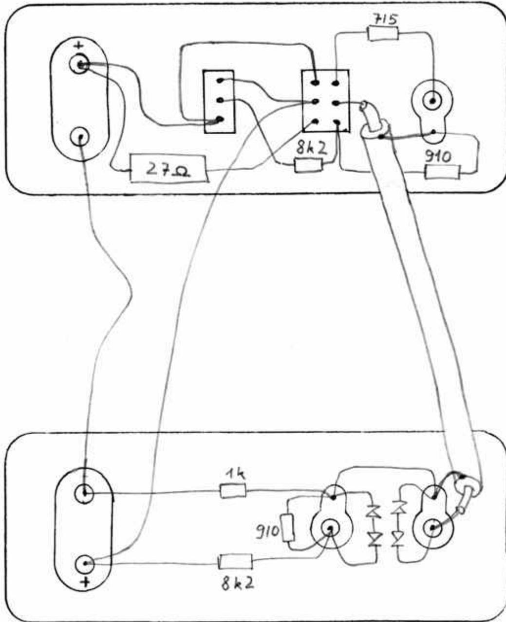
Figure 5. Connection plan for Measuring box
