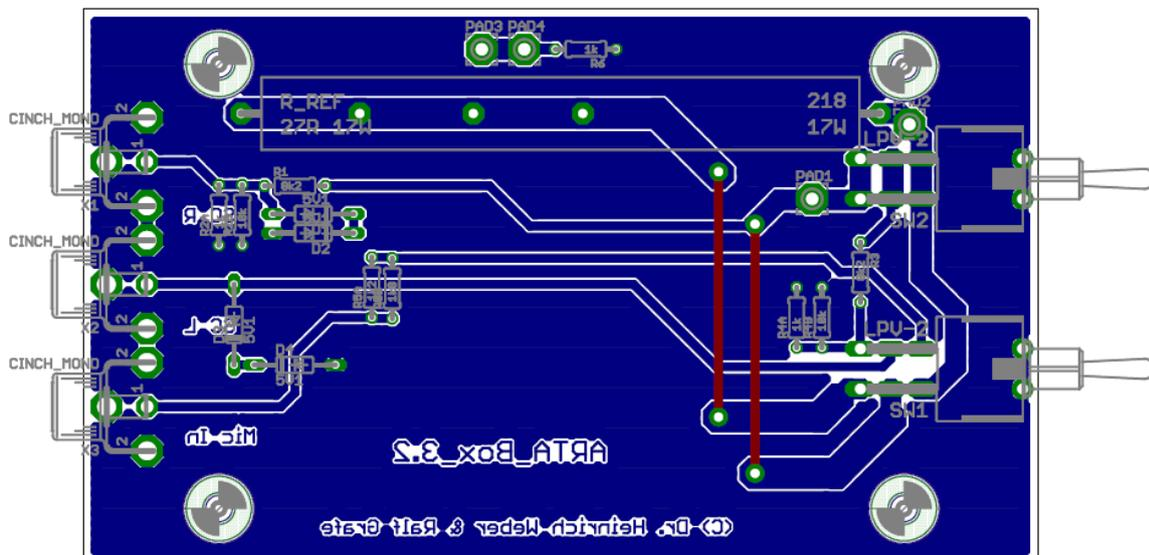
Figure 8. Component side of the PCB for the ARTA-MeasuringBox
