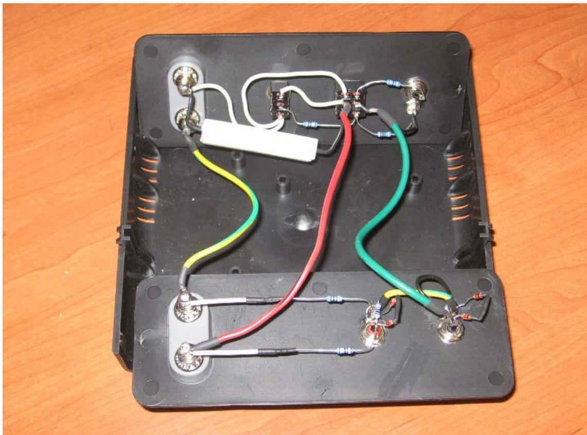
Figure 3. The picture of connections inside the MeasuringBox
