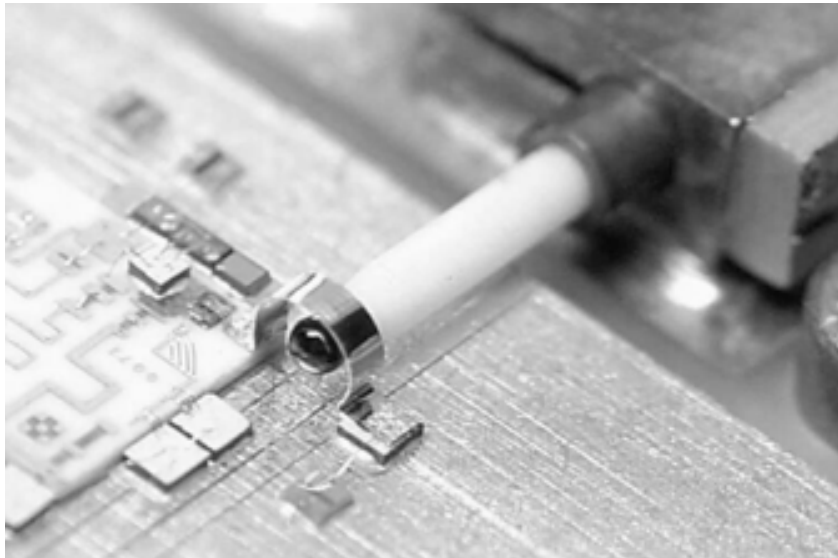
Figure 7.22 YIG sphere mounted at the end of a ceramic rod and coupled to the RF circuit via a loop band (courtesy VHF Communications magazine).
